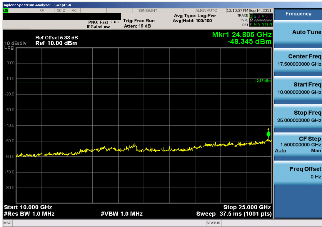
Plot 6-17. Conducted Spurious Plot (Bluetooth, 1Mbps – Ch. 0)
