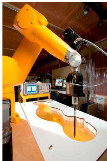
Figure 3-2 DASY4 SAR Measurement System
