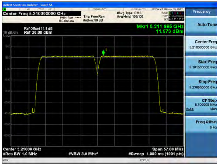
64QAM UNII 1 BAND PSD_5210 MHz
