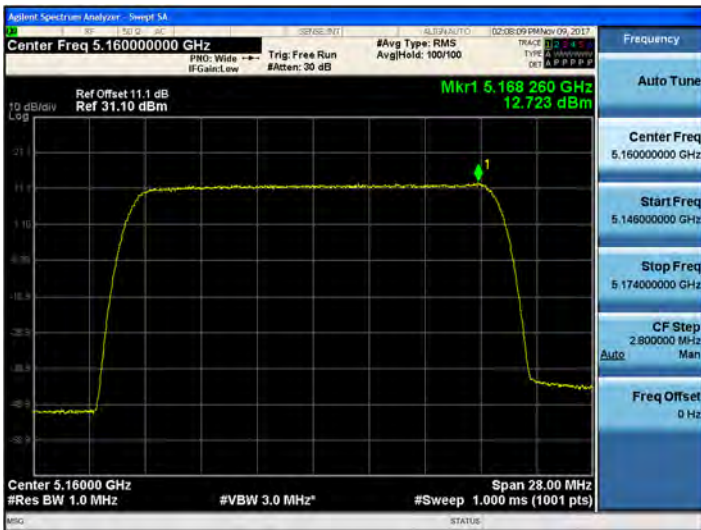
64QAM UNII 1 BAND PSD_5160 MHz
