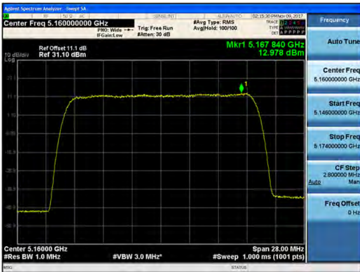
16QAM UNII 1 BAND PSD_5160 MHz
