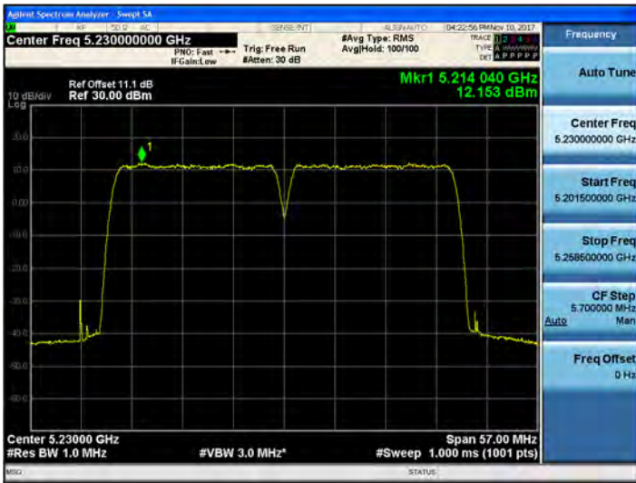
16QAM UNII 1 BAND PSD_5230 MHz
