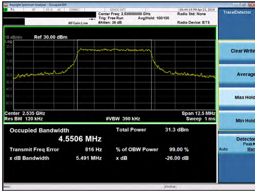
Plot 7-88. Occupied Bandwidth Plot (Band 7 - 5.0MHz QPSK - Full RB Configuration)
