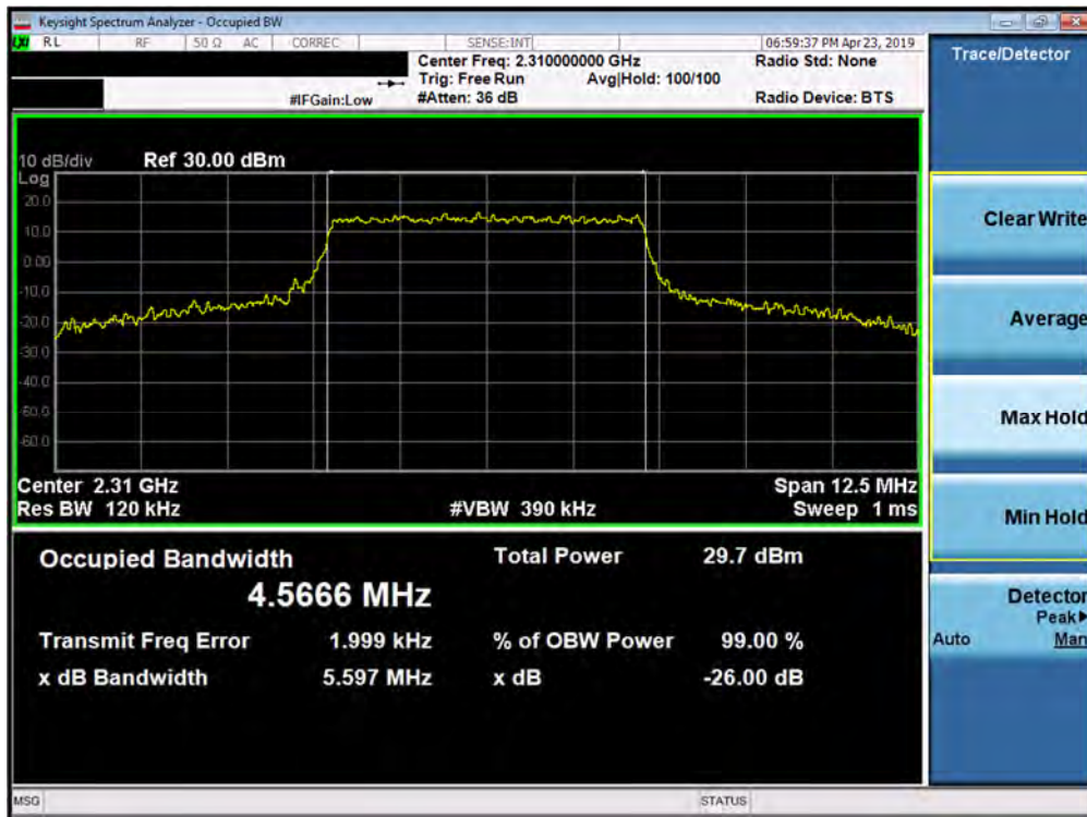
Plot 7-84. Occupied Bandwidth Plot (Band 30 - 5.0MHz 64-QAM - Full RB Configuration)
