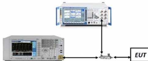
Figure 7-4. Test Instrument & Measurement Setup
