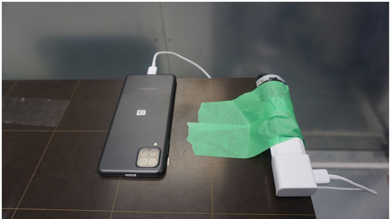
Conducted Test Configuration 3 and 4: Charging (with travel adapter) and Video + Audio playback from internal memory data + Charging (with travel adapter)
