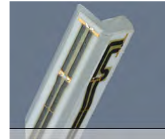
Figure 4-1 E-field Free-space Probe
