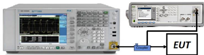
Figure 7-7. Test Instrument & Measurement Setup
