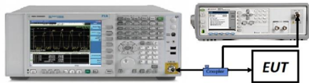
Figure 7-2. Test Instrument & Measurement Setup
