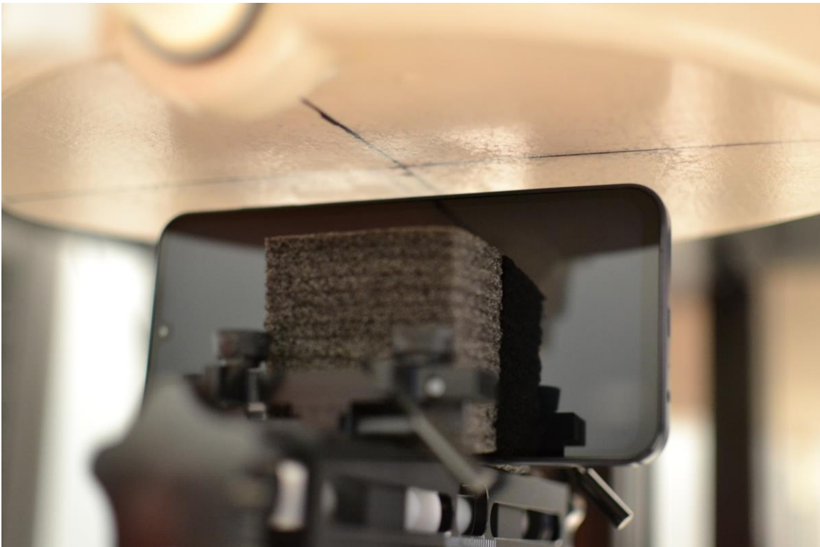
SAR Test Setup Photo 12 – Hotspot, Right Edge at 10mm
