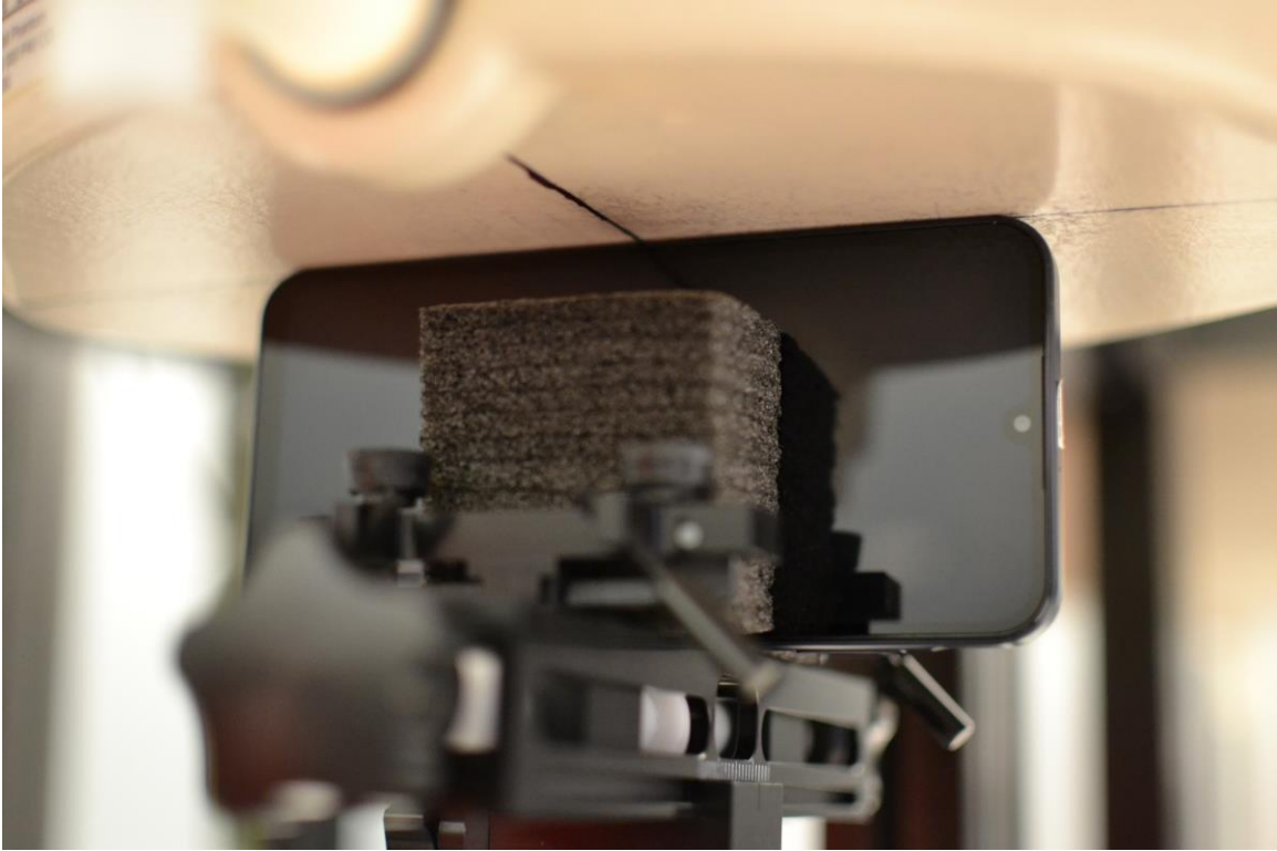
SAR Test Setup Photo 14 – Phablet, Left Edge at 0mm
