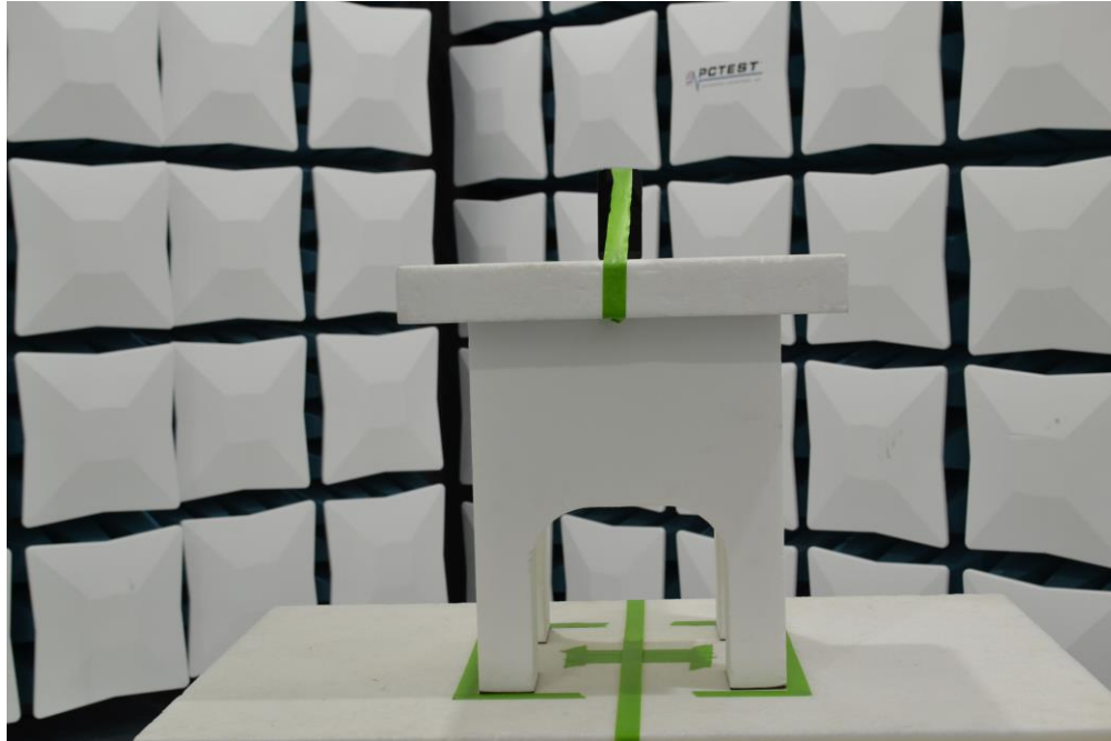
Figure 3. Test Setup – Z Position – 1GHz-18GHz
