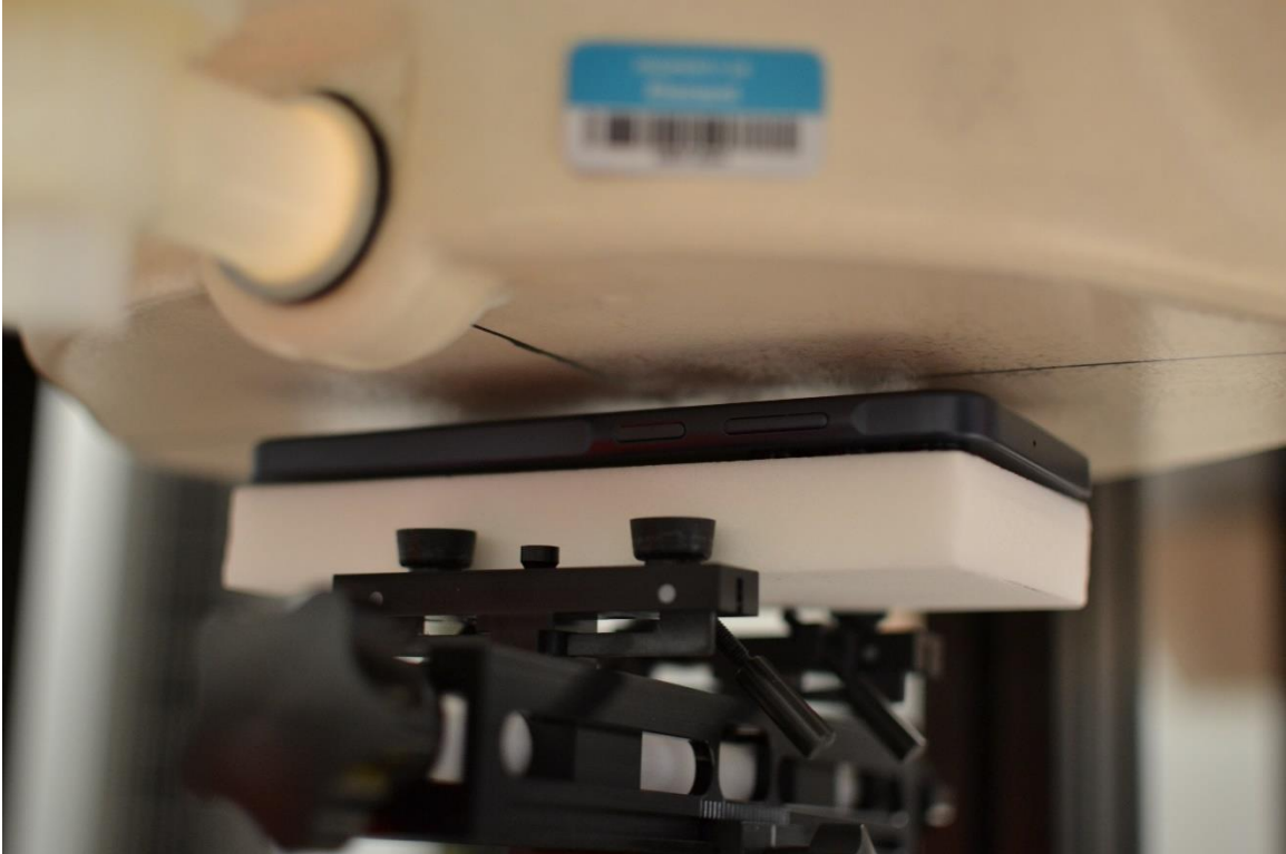
SAR Test Setup Photo 7 – Hotspot, Front Side at 10mm
