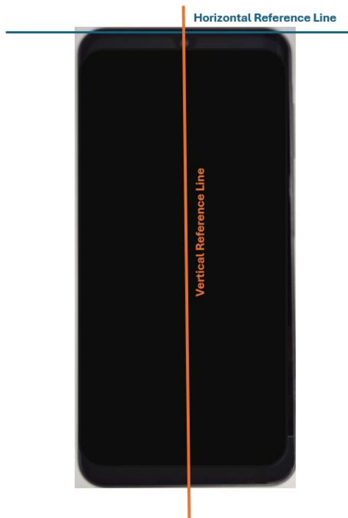
Figure Y SAR Test Setup – Reference Lines
