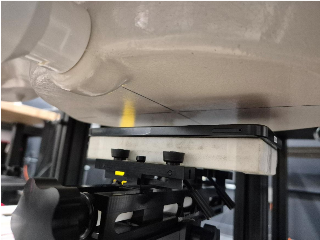
Figure F SAR Test Setup – Body-worn – Back 17mm
