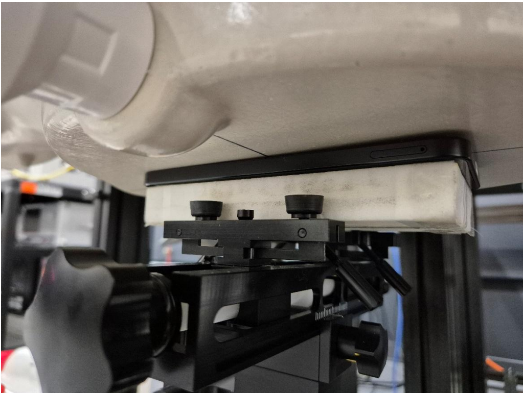
Figure K SAR Test Setup – Phablet – Back 0mm
