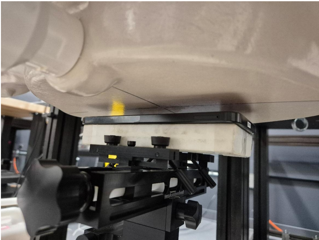
Figure G SAR Test Setup – Body-worn/Phablet – Back 13mm
