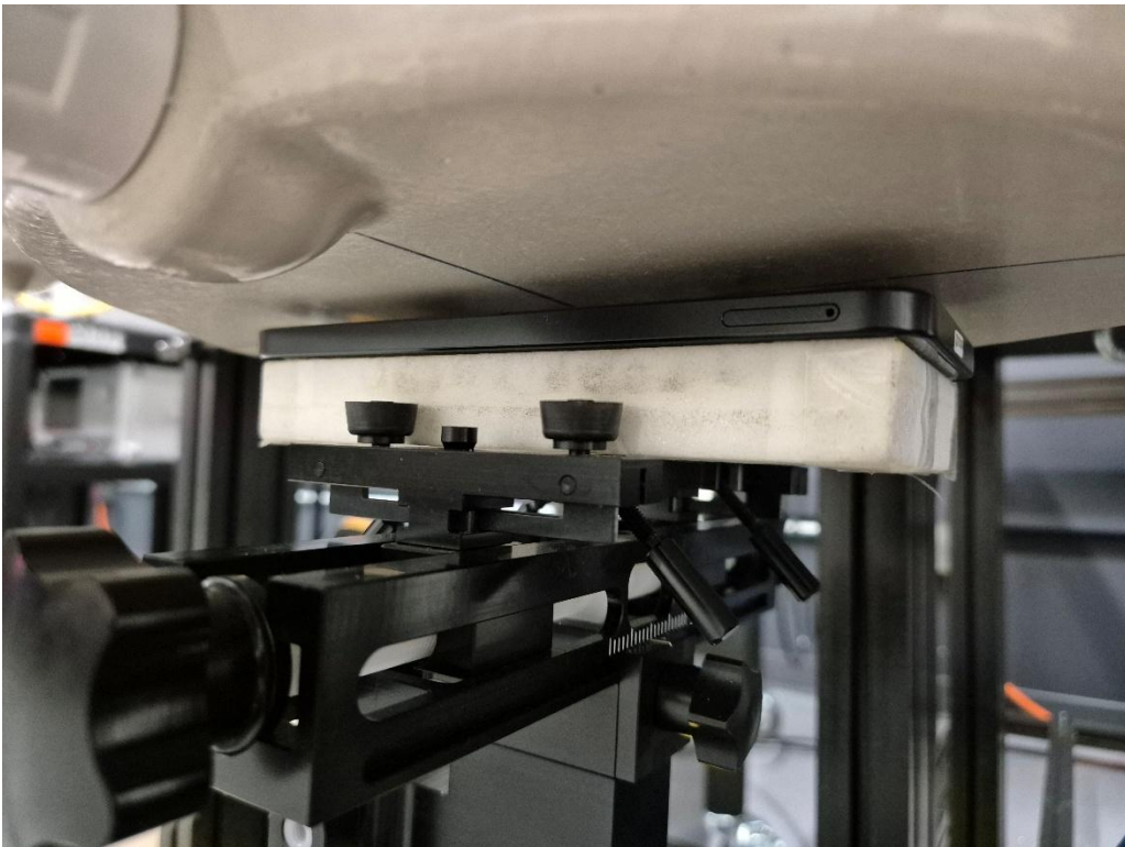
Figure I SAR Test Setup – Body-worn / Hotspot – Back 5mm
