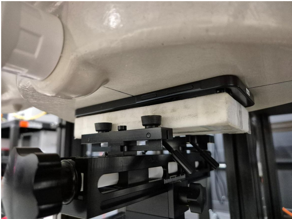
Figure M SAR Test Setup – Phablet – Front 0mm
