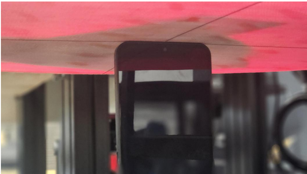
Figure W SAR Test Setup – Phablet on ELI – Top 0mm
