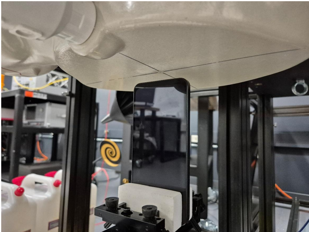
Figure Q SAR Test Setup – Hotspot – Bottom 10mm
