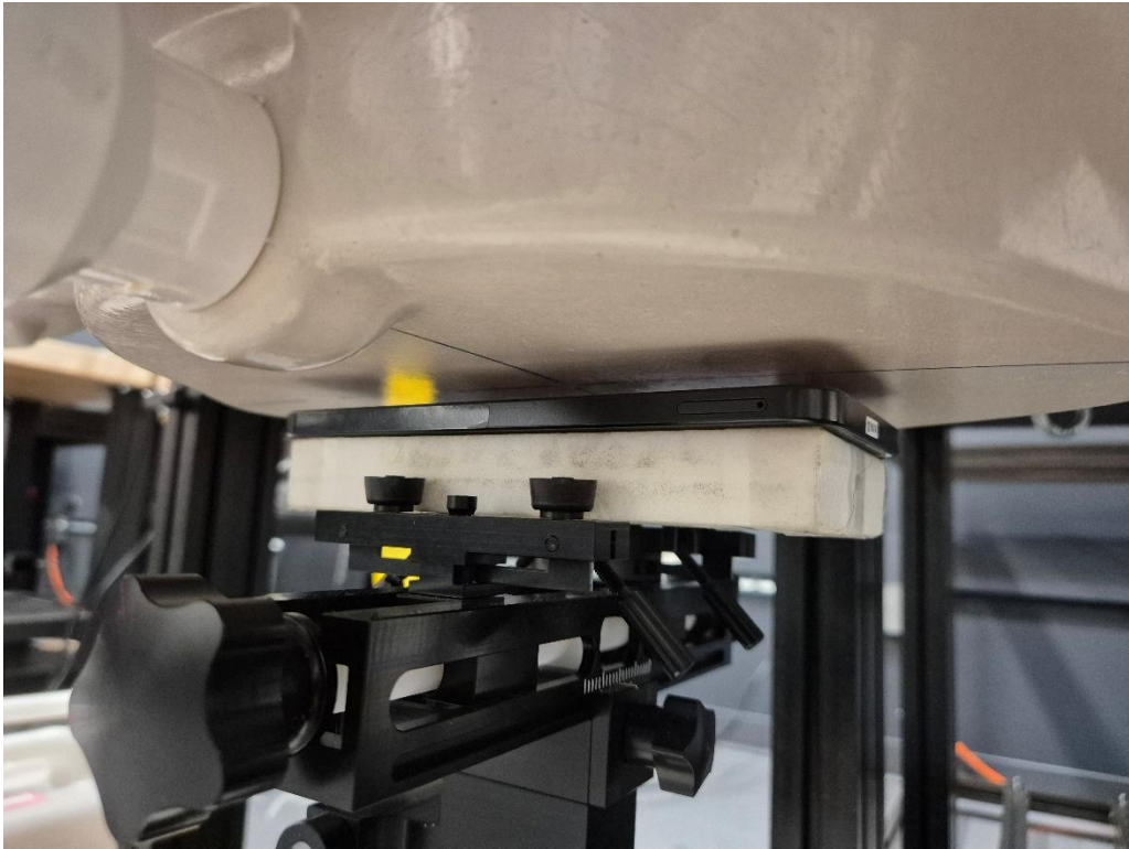
Figure H SAR Test Setup – Hotspot – Back 10mm
