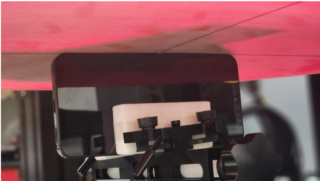
Figure X SAR Test Setup – Phablet on ELI – Left 0mm
