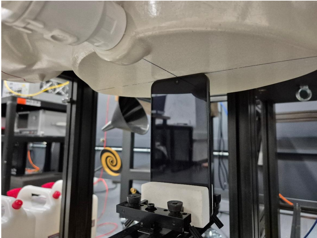
Figure P SAR Test Setup – Phablet – Top 0mm
