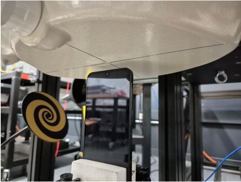
Figure N SAR Test Setup – Hotspot – Top 11mm
