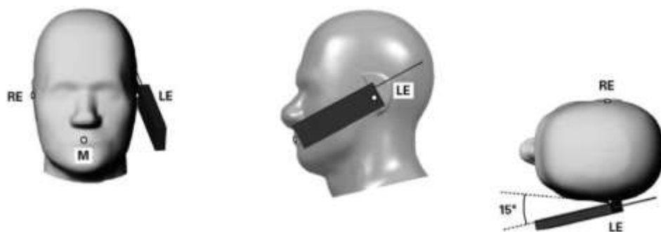
Figure 8.5. Tilt 15° position of the wireless device
