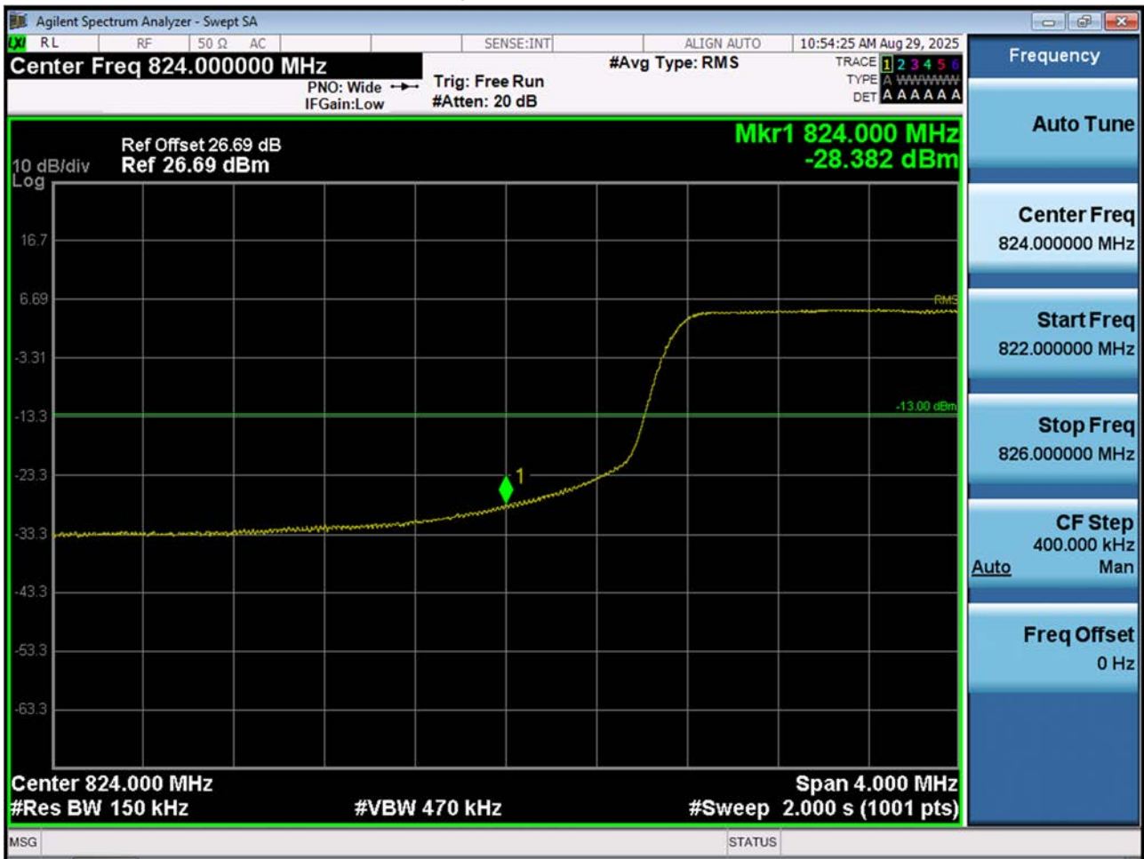
LTE B26_ Lower Band Edge Plot (15 M BW Ch.26865 QPSK_RB75_Offset 0)
