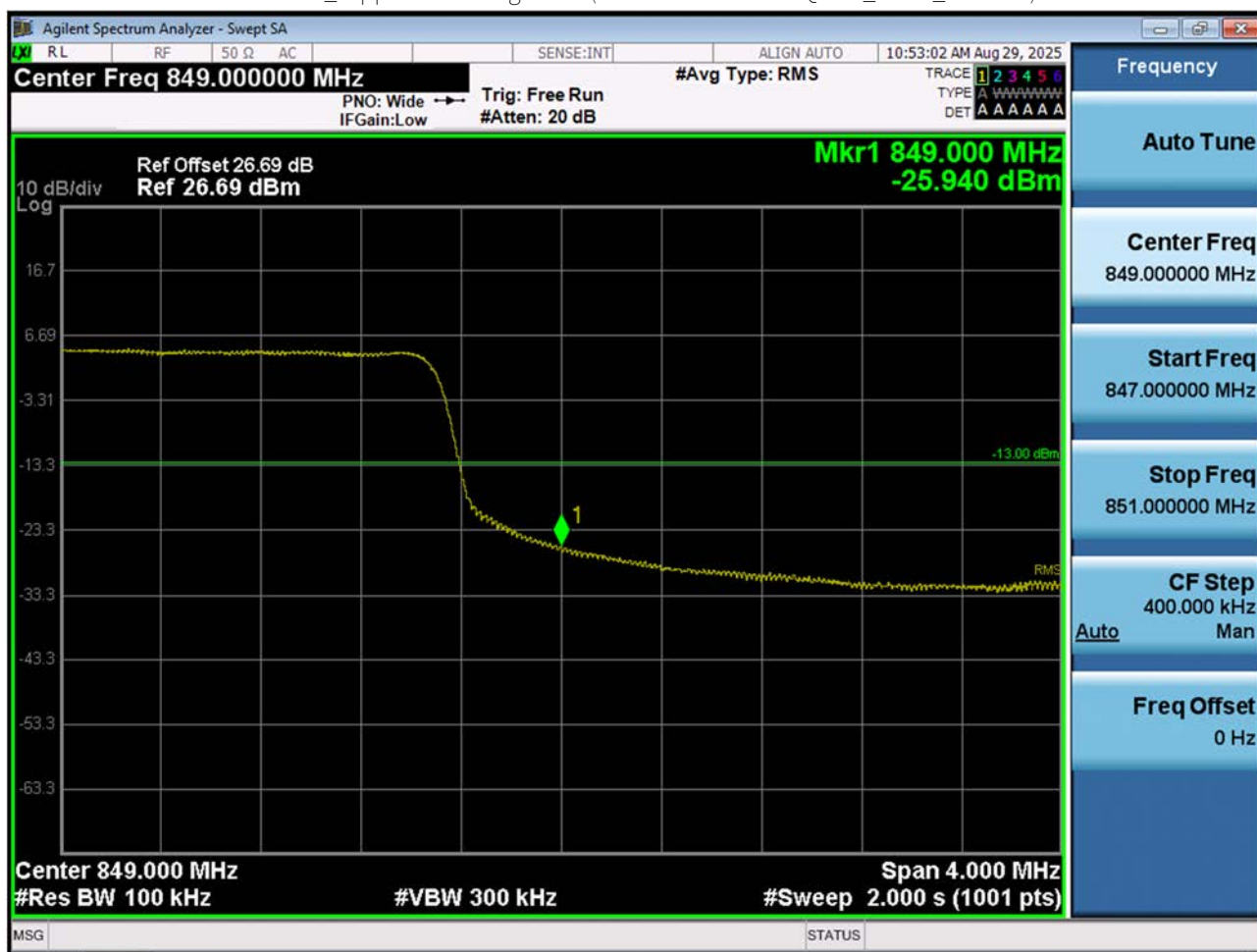
LTE B26_ Upper Band Edge Plot (10 M BW Ch.26990 QPSK_RB50_Offset 0)
