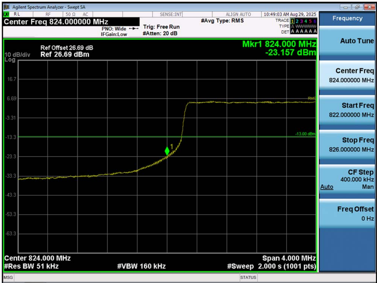
LTE B26_ Lower Band Edge Plot (5 M BW Ch.26815 QPSK_RB25_Offset 0)
