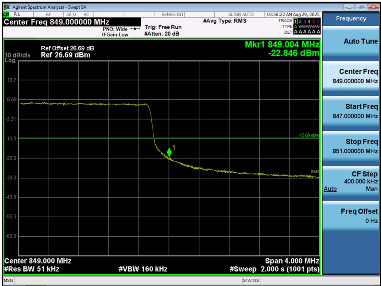
LTE B26_ Upper Band Edge Plot (5 M BW Ch.27015 QPSK_RB25_Offset 0)
