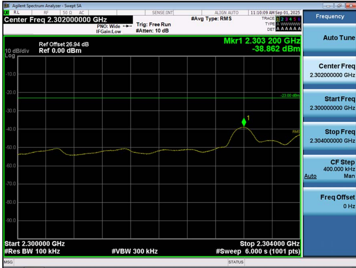
LTE B30_5 M_Band Edge(2300MHz-2304MHz)_Low_QPSK_1RB
