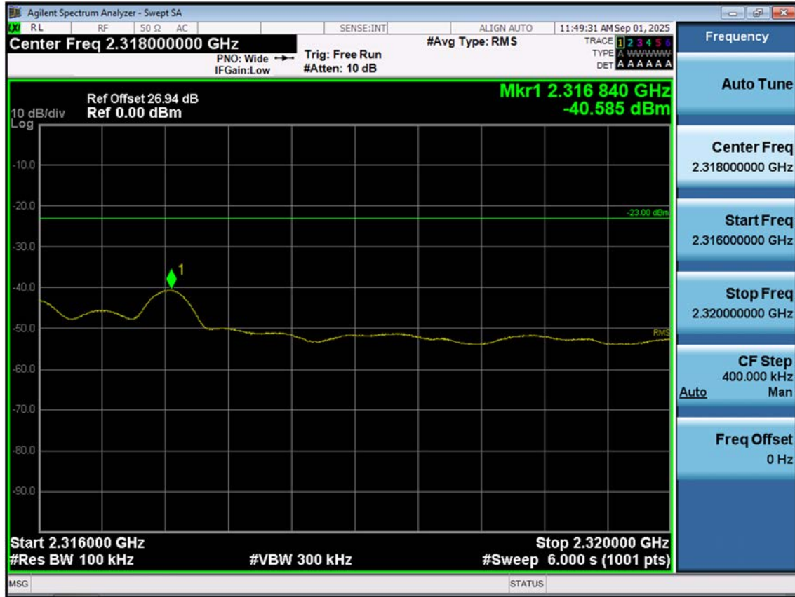
LTE B30_5 M_Band Edge(2316MHz-2320MHz)_High_QPSK_1RB
