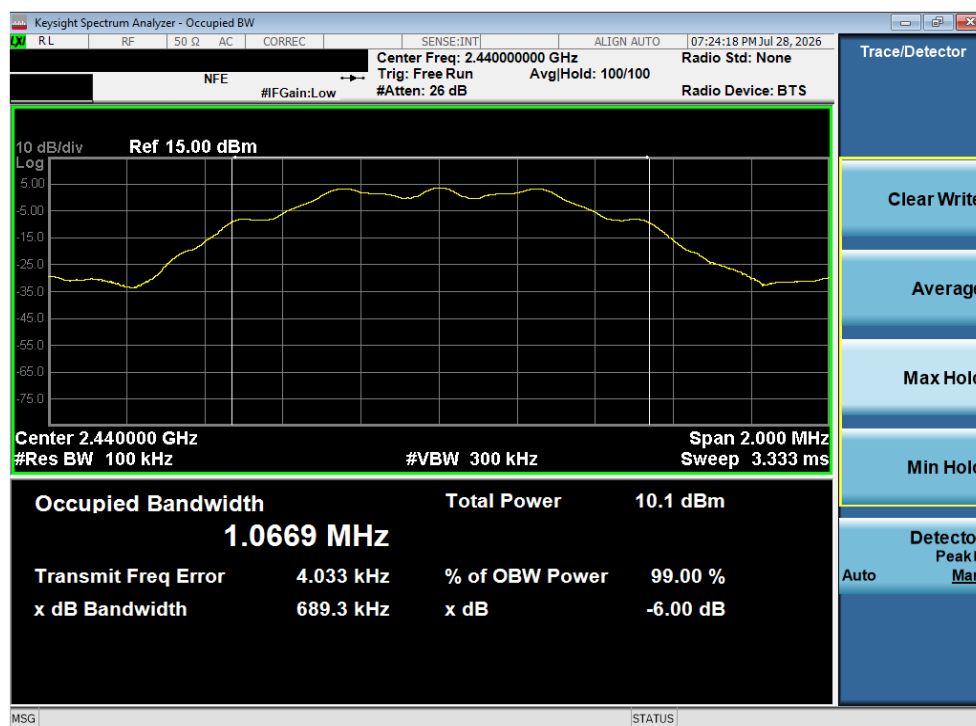
Plot 7-2. 6dB Bandwidth Plot (Bluetooth (LE), 125kbps – Ch. 17)
