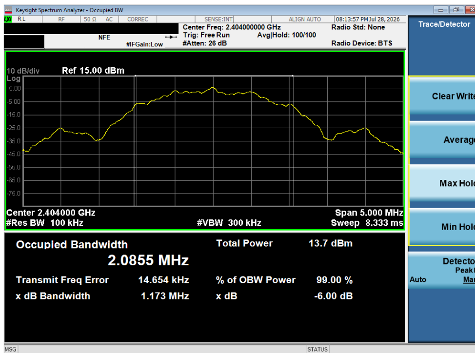
Plot 7-10. 6dB Bandwidth Plot (Bluetooth (LE), 2Mbps – Ch. 0)
