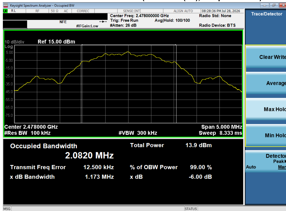
Plot 7-12. 6dB Bandwidth Plot (Bluetooth (LE), 2Mbps – Ch. 36)
