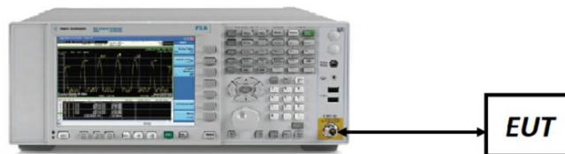
Figure 7-5. Test Instrument & Measurement Setup
