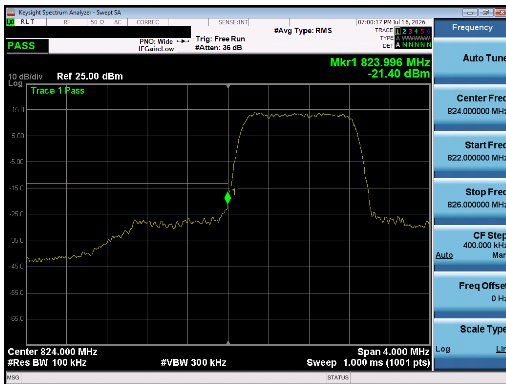
Plot 7-23. Lower Band Edge Plot (LTE Band 26/5 – 1.4MHz QPSK – Full RB)
