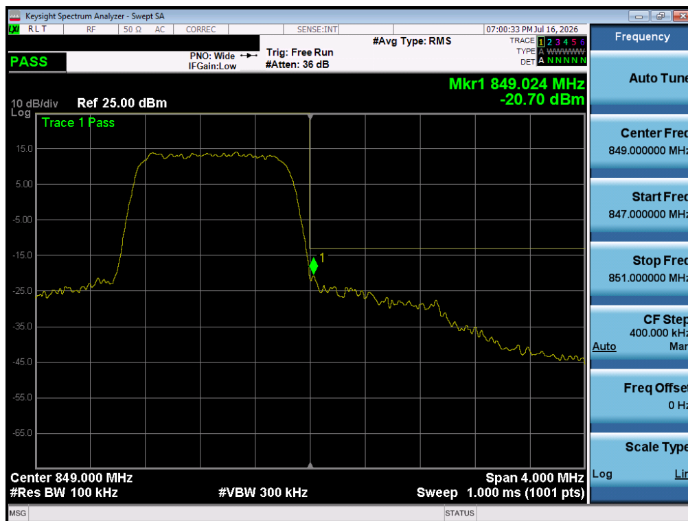
Plot 7-24. Upper Band Edge Plot (LTE Band 26/5 – 1.4MHz QPSK – Full RB)
