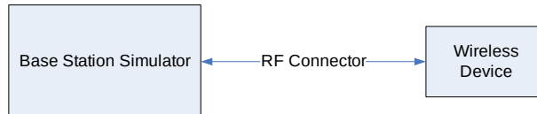
Figure 9-2 Power Measurement Setup
