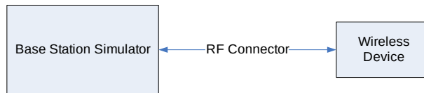
Figure 9-1 Power Measurement Setup
