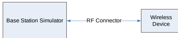
Figure 9-2 Power Measurement Setup
