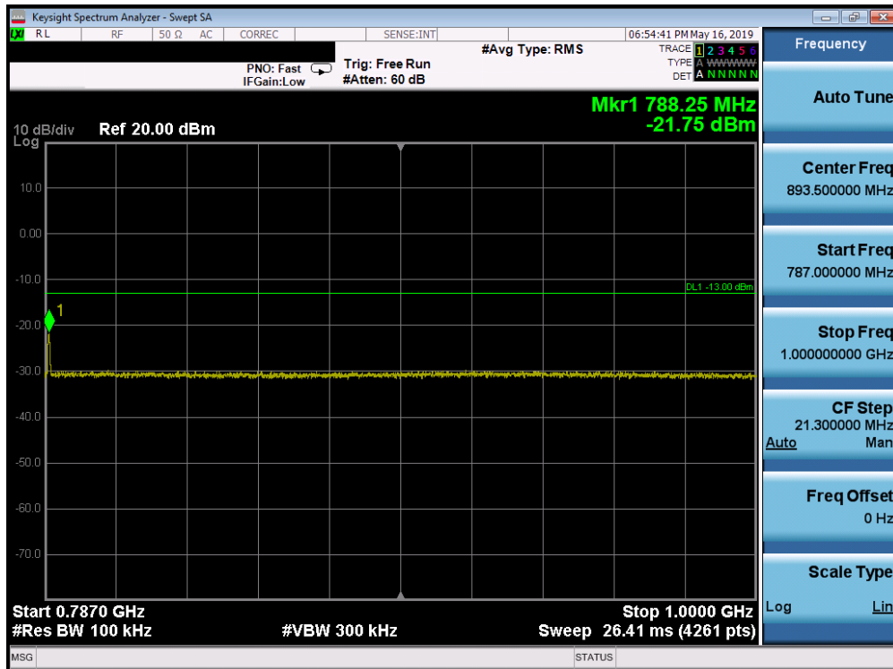
Plot 7-140. Conducted Spurious Plot (Band 13 - 5.0MHz QPSK - RB Size 1, RB Offset 0 - Mid Channel)
