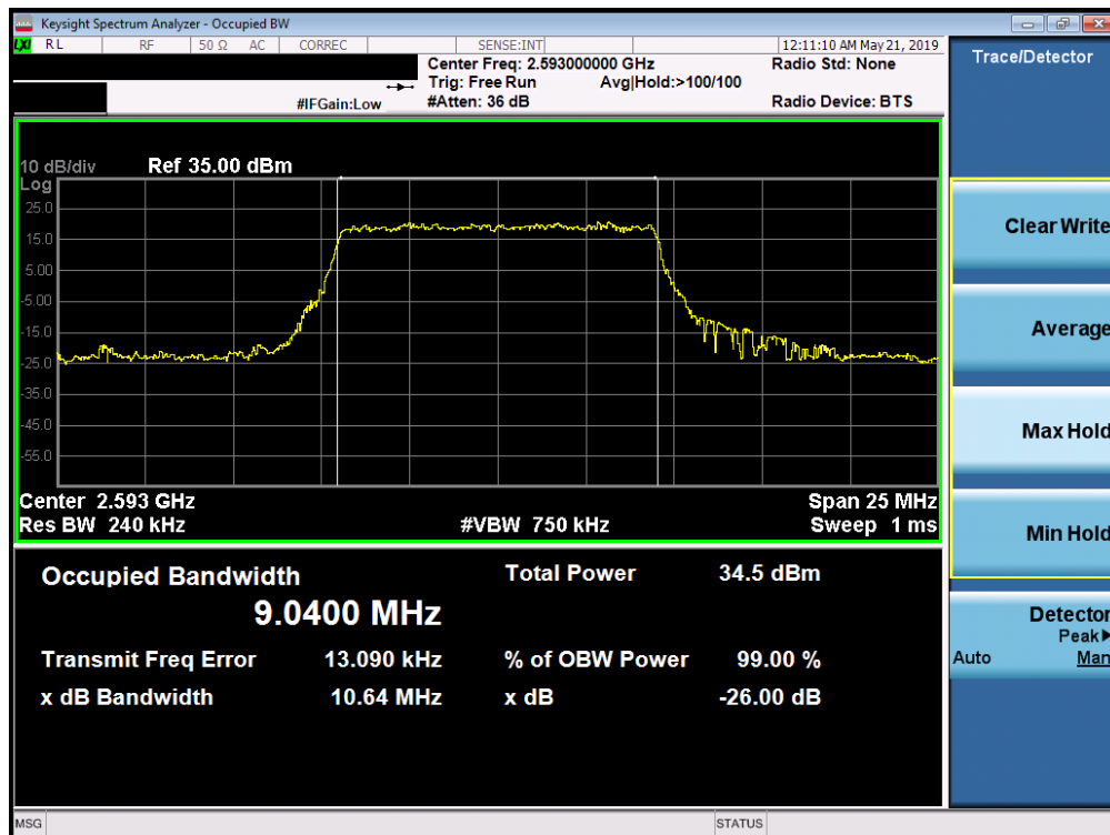
Plot 7-97. Occupied Bandwidth Plot (Band 41 PC2 - 10.0MHz QPSK - Full RB Configuration)
