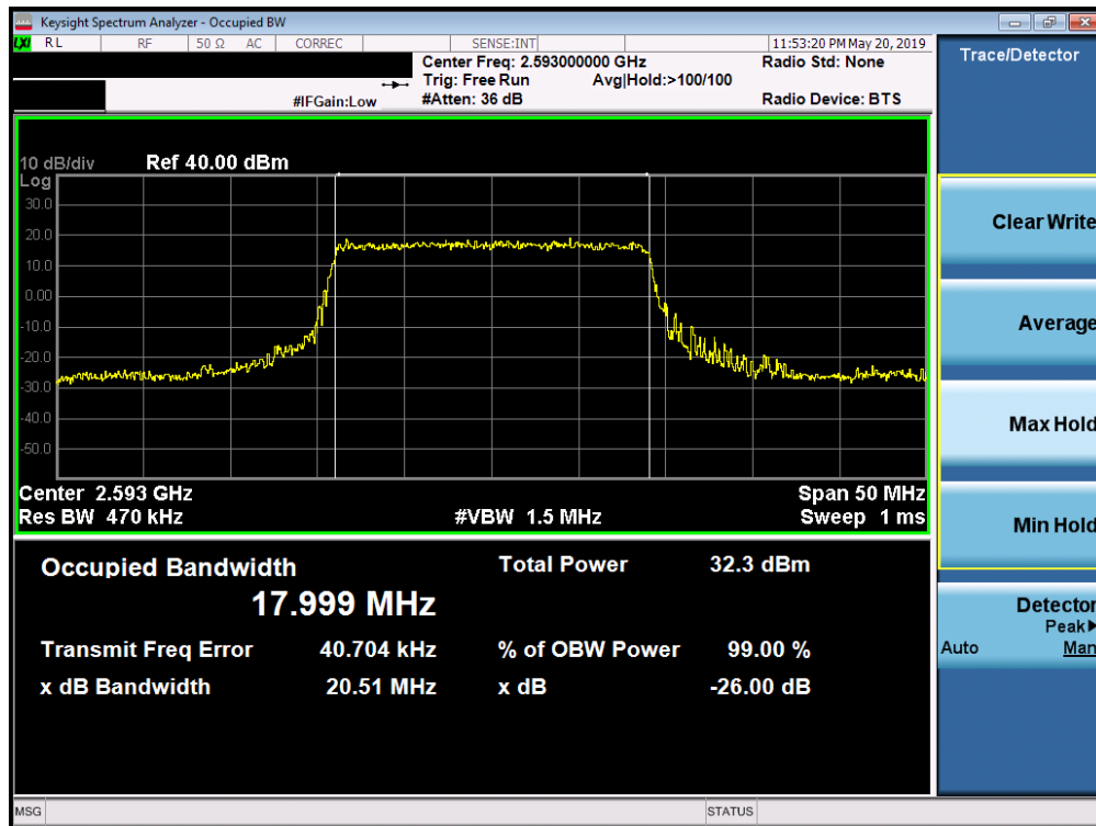
Plot 7-105. Occupied Bandwidth Plot (Band 41 PC2 - 20.0MHz 64-QAM - Full RB Configuration)
