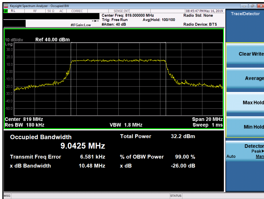
Plot 7-13. Occupied Bandwidth Plot (LTE Band 26, 10MHz 16-QAM – RB Size 50)
