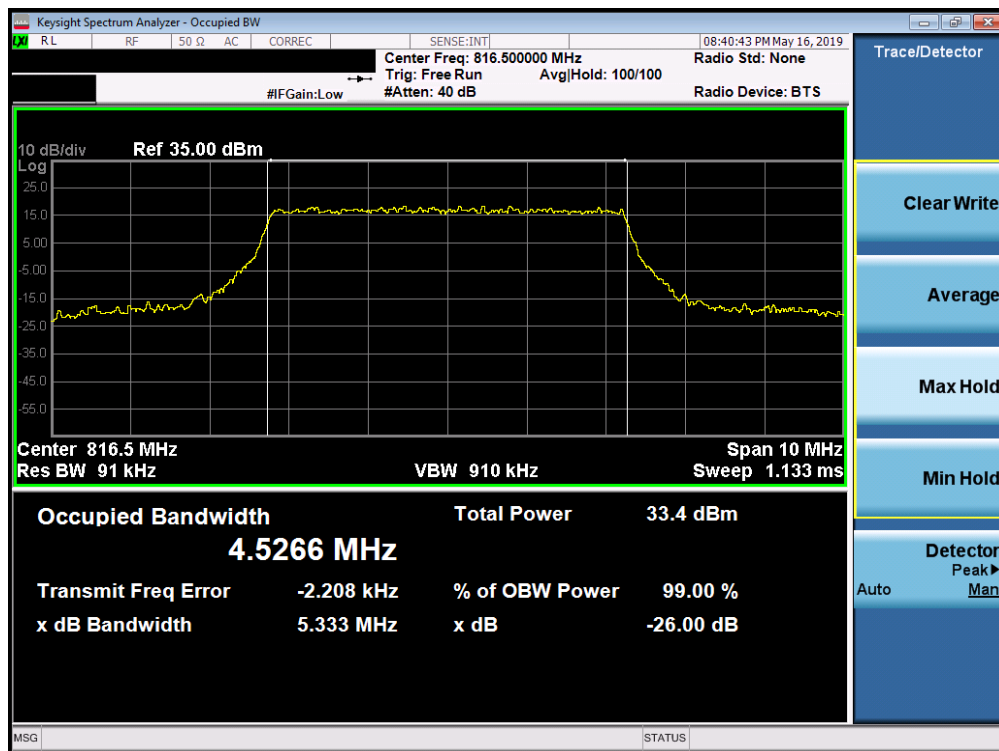
Plot 7-9. Occupied Bandwidth Plot (LTE Band 26, 5MHz QPSK – RB Size 25– Low Channel)
