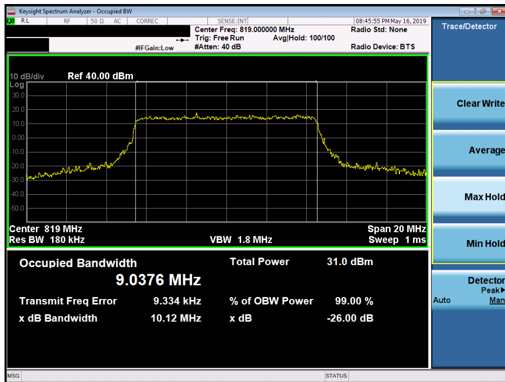
Plot 7-14. Occupied Bandwidth Plot (LTE Band 26, 10MHz 64-QAM – RB Size 50)
