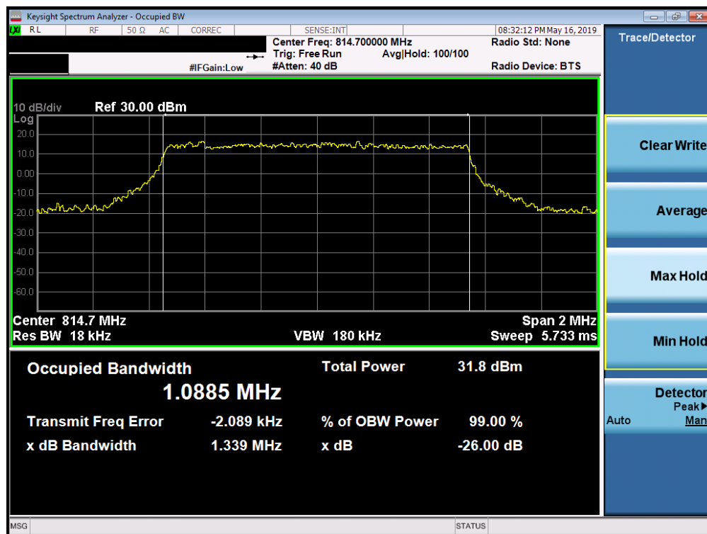
Plot 7-4. Occupied Bandwidth Plot (LTE Band 26, 1.4MHz 16-QAM – RB Size 6– Low Channel)
