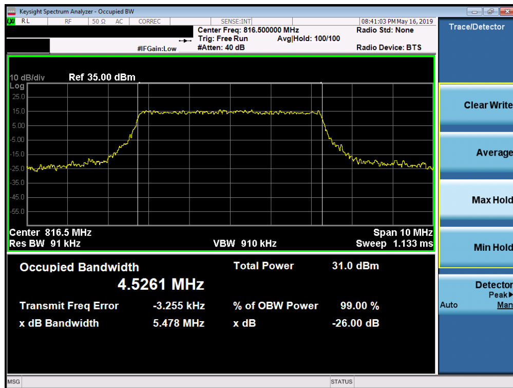
Plot 7-11. Occupied Bandwidth Plot (LTE Band 26, 5MHz 64-QAM – RB Size 25– Low Channel)
