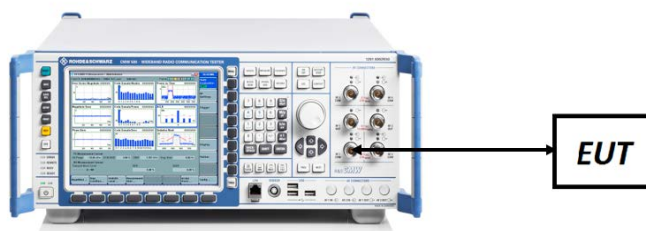
Figure 7-4. ERP/EIRP Measurement Setup
