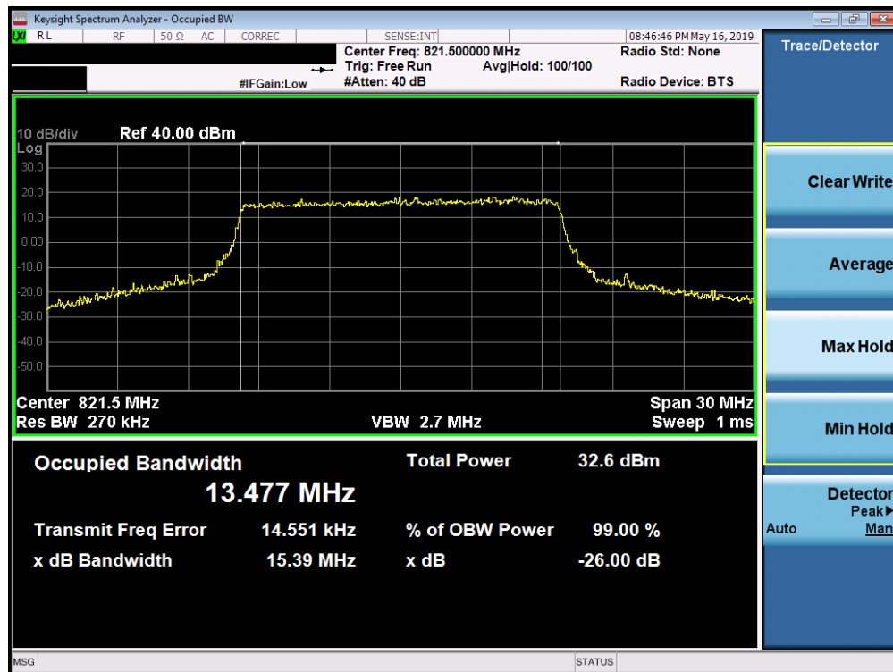
Plot 7-16. Occupied Bandwidth Plot (LTE Band 26, 15MHz 16-QAM – RB Size 75)
