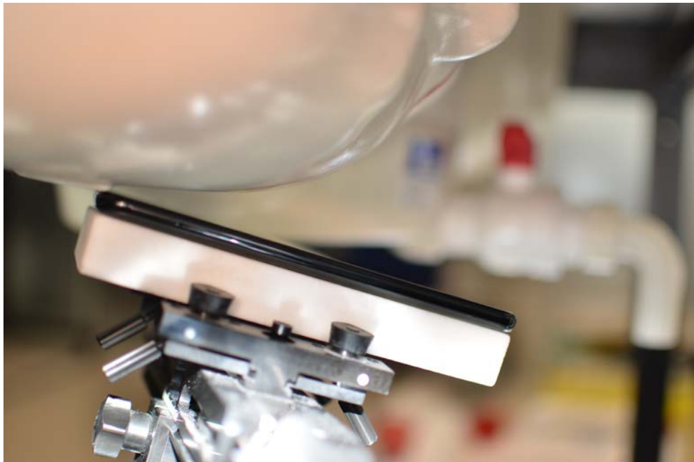
SAR Test Setup Photo 2: Right Tilt
