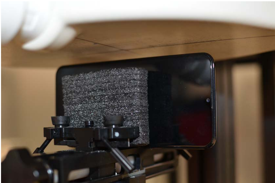
SAR Test Setup Photo 18: Left Edge at 1.0 cm
