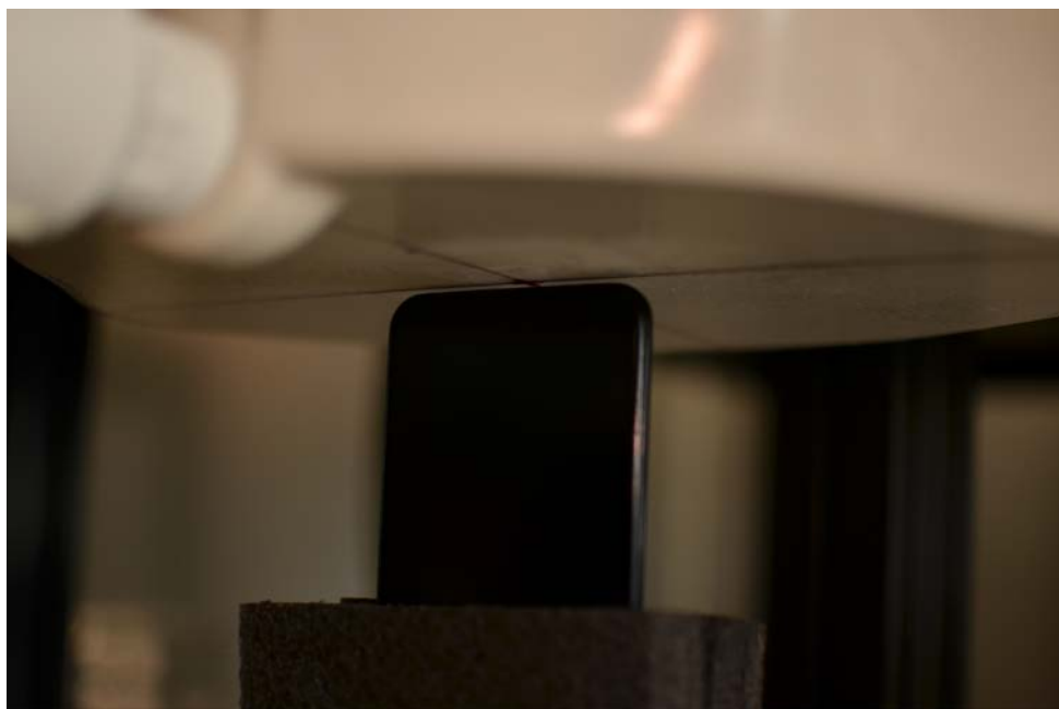
SAR Test Setup Photo 14: Bottom Edge at 0.2 cm
