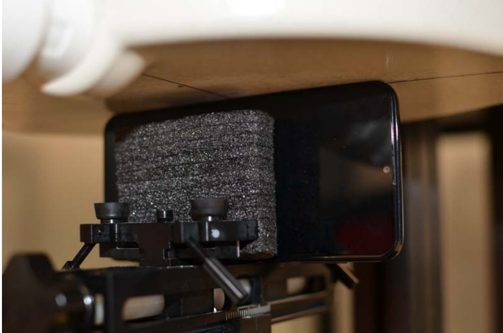
SAR Test Setup Photo 19: Left Edge at 0.0 cm
