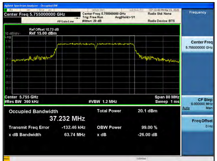
802.11ac_VHT40 UNII 3 BAND 26dB Bandwidth (CH 151)
