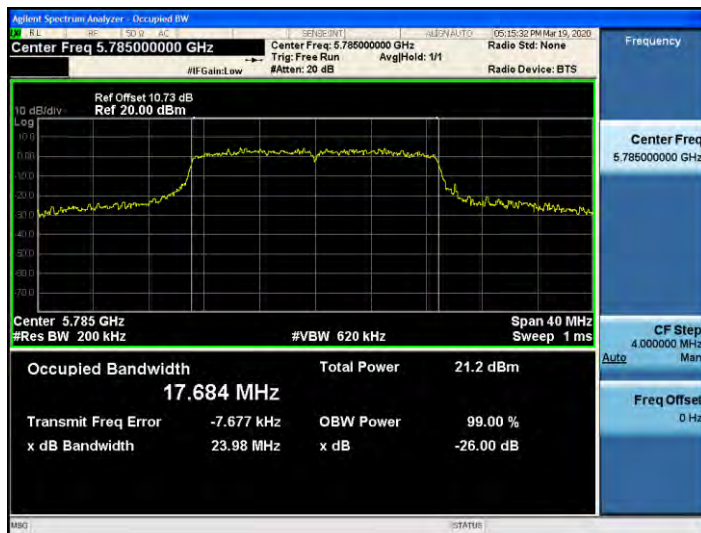
802.11ac_VHT20 UNII 3 BAND 26dB Bandwidth(CH 157)
