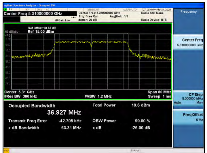
802.11ac_VHT40 UNII 3 BAND 26dB Bandwidth (CH 151)
