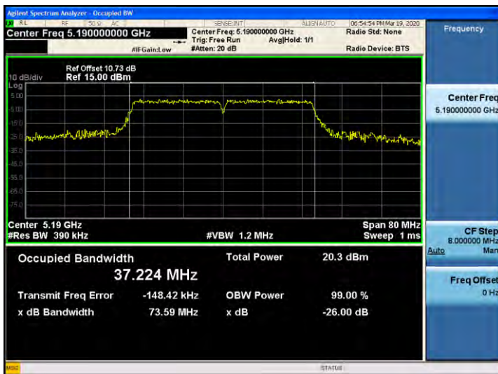
802.11ac_VHT40 UNII 2C BAND 26dB Bandwidth(CH 142)
