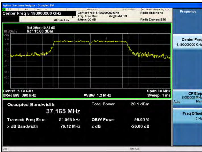
802.11n_HT40 UNII 2C BAND 26dB Bandwidth(CH 142)
