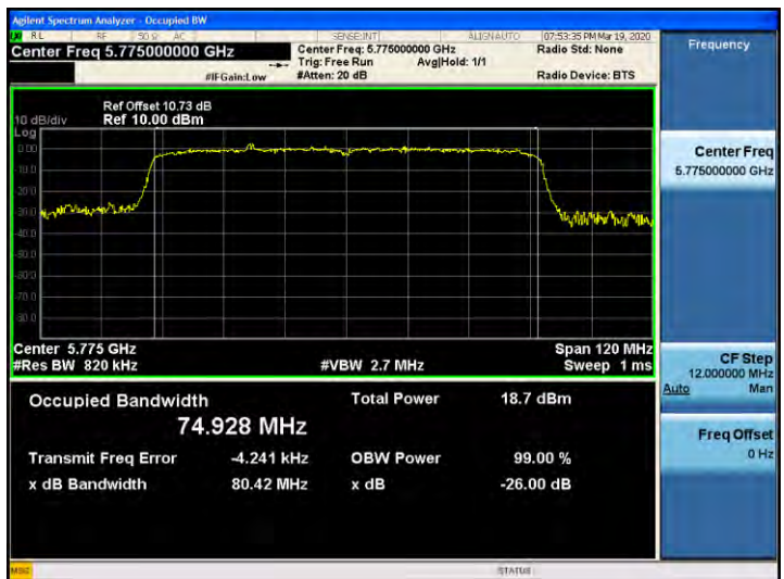
802.11ac_VHT80 UNII 3 BAND 26dB Bandwidth (CH 155)
