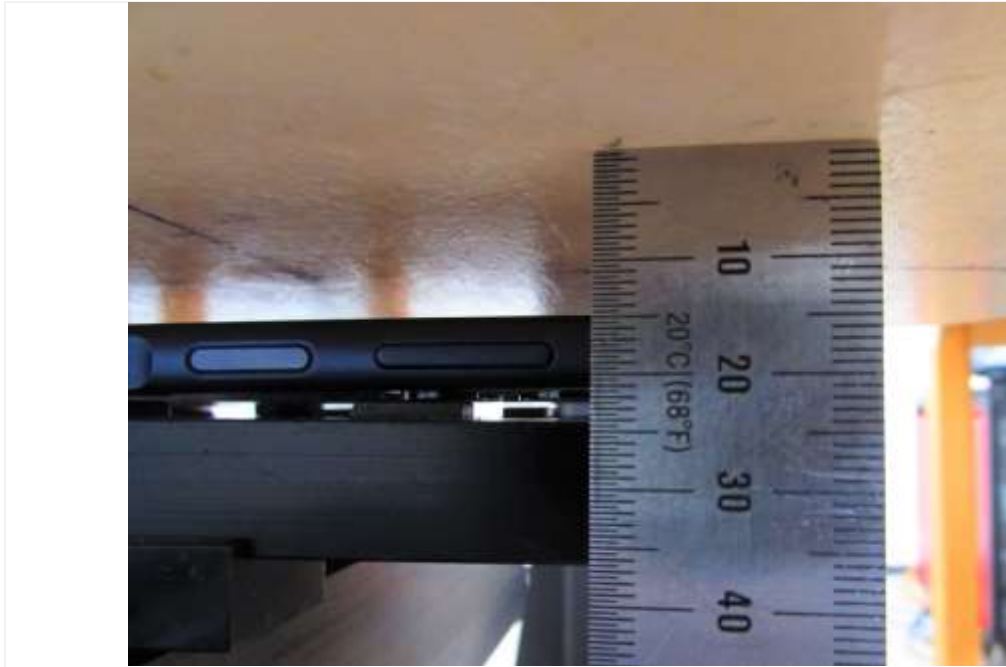
Distance of 15 mm from the EUT
