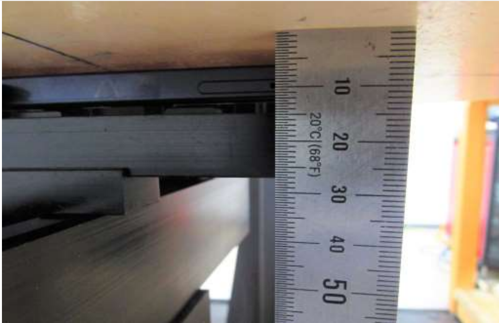
Distance of 6 mm from the EUT
