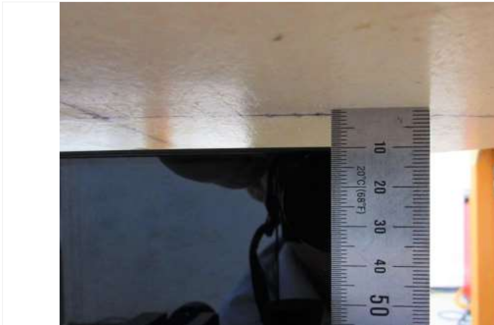
Distance of 10 mm from the EUT
