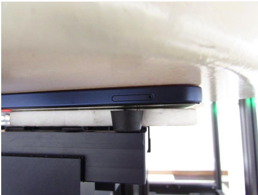
Distance of 0 mm from the EUT
