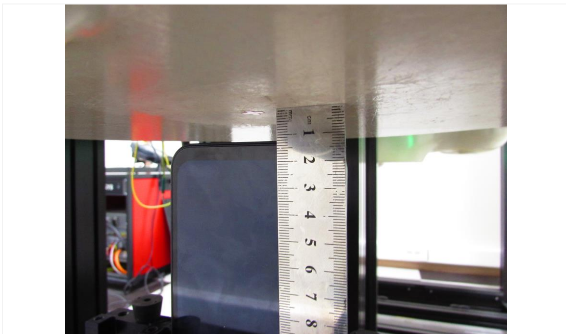
Distance of 12 mm from the EUT
