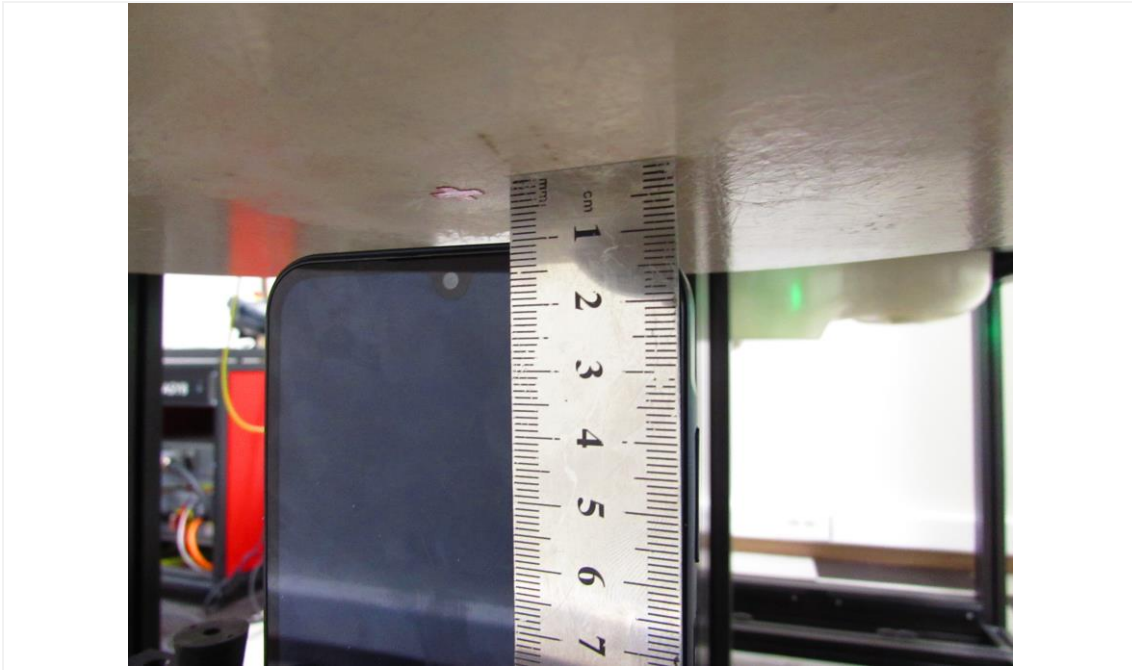
Distance of 10 mm from the EUT
