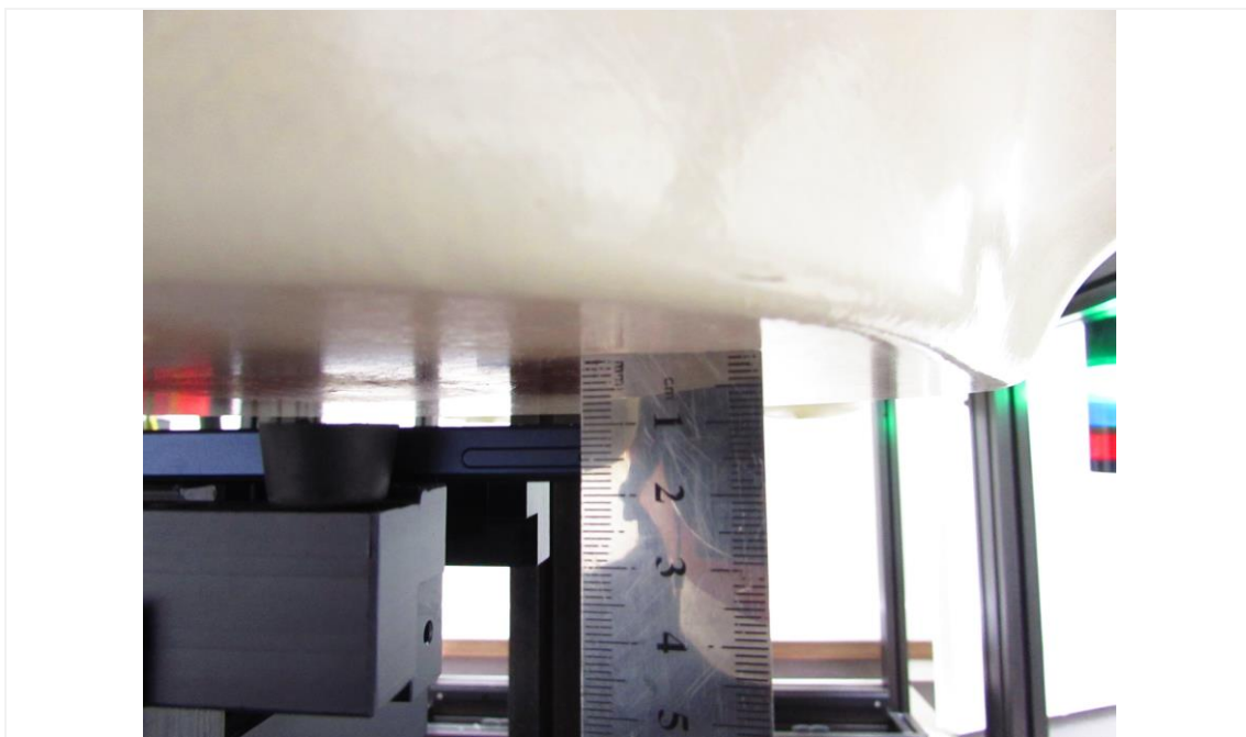
Distance of 10 mm from the EUT
