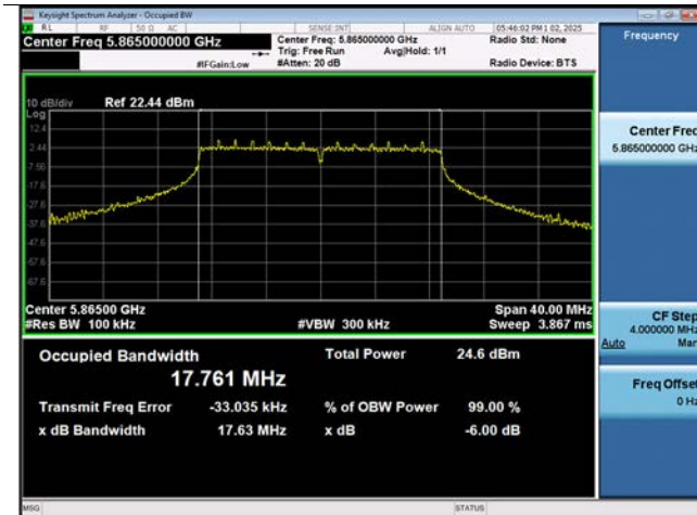
802.11ac(VHT40) 6 dB Bandwidth (CH 175)
