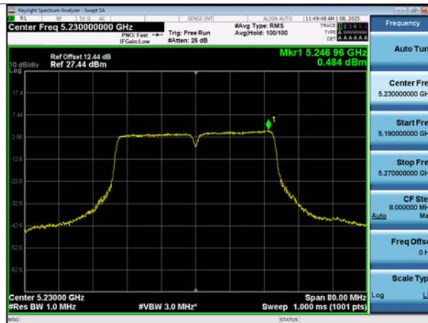
Bandwidth 80M, 802.11ac(VHT80) (Ch. 122)
