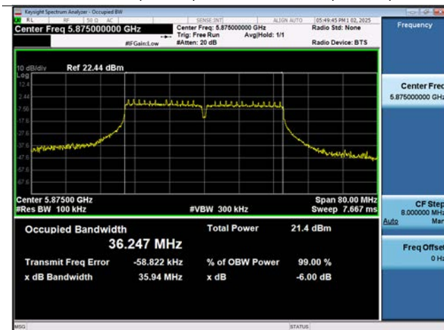
802.11ac(VHT40) 6 dB Bandwidth (CH 175)
