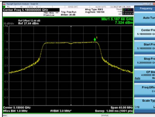
Bandwidth 40M, 802.11ac(VHT40) (Ch. 46)
