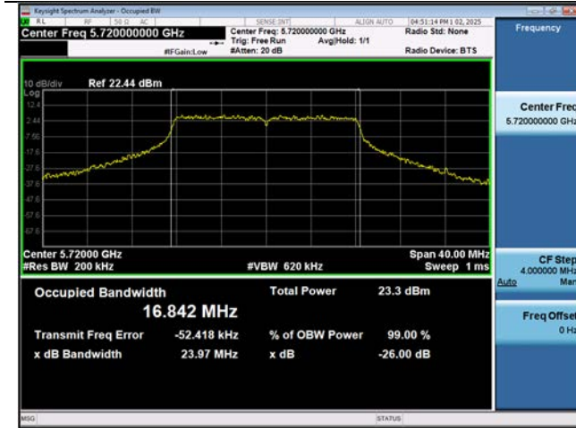
802.11ac(VHT20) 26 dB Bandwidth (CH 60)
