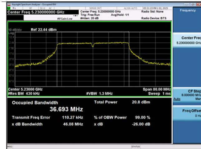
802.11ac(VHT40) 26 dB Bandwidth (CH 46)
