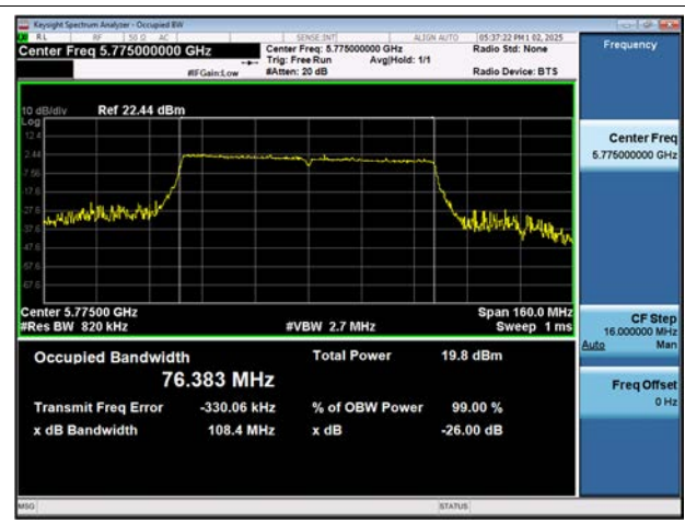
802.11ac(VHT80) 26 dB Bandwidth (CH 155)
