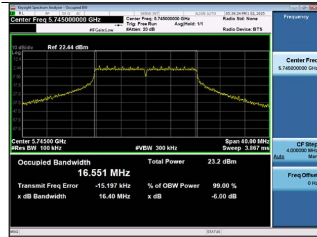
802.11ac(VHT20) 6 dB Bandwidth (CH 173)
