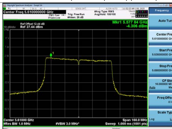
Bandwidth 80M, 802.11ac(VHT80) (Ch. 122)
