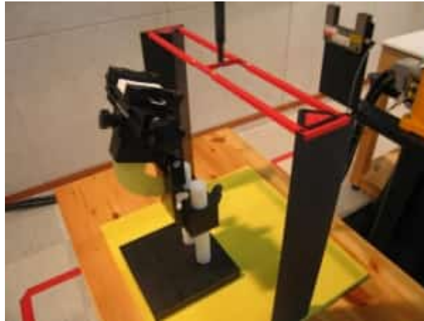
Figure 2. HAC Phantom & Device Holder
