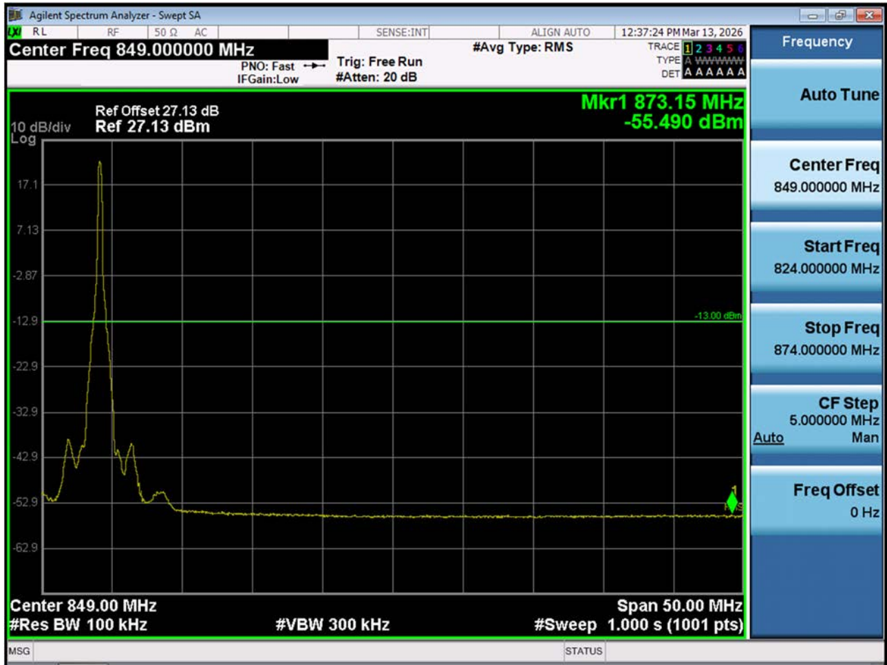
LTE B26_ Mid Band Edge Plot (15 M BW Ch.26765 QPSK RB 1, Offset74)
