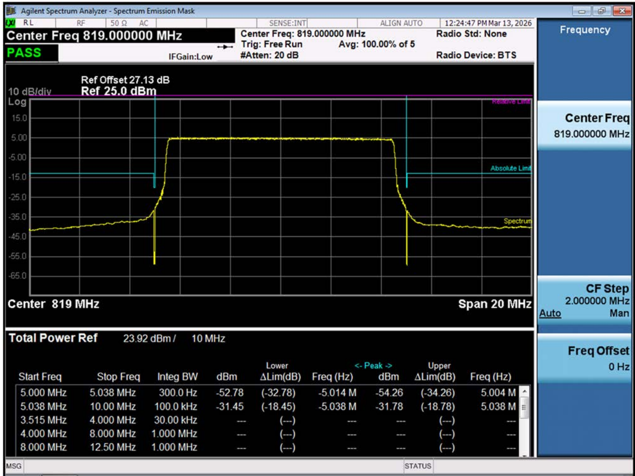
LTE B26_ Low Channel Edge Plot (10 M BW Ch.26740 QPSK_RB50_Offset 0)
