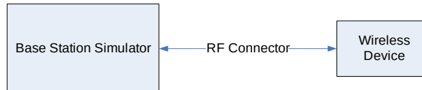
Figure 9-1 Power Measurement Setup
