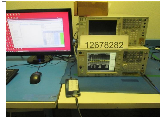
RF ANTENNA PORT CONDUCTED
