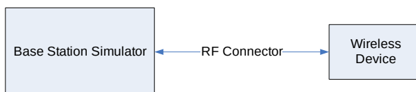
Figure 9-1 Power Measurement Setup
