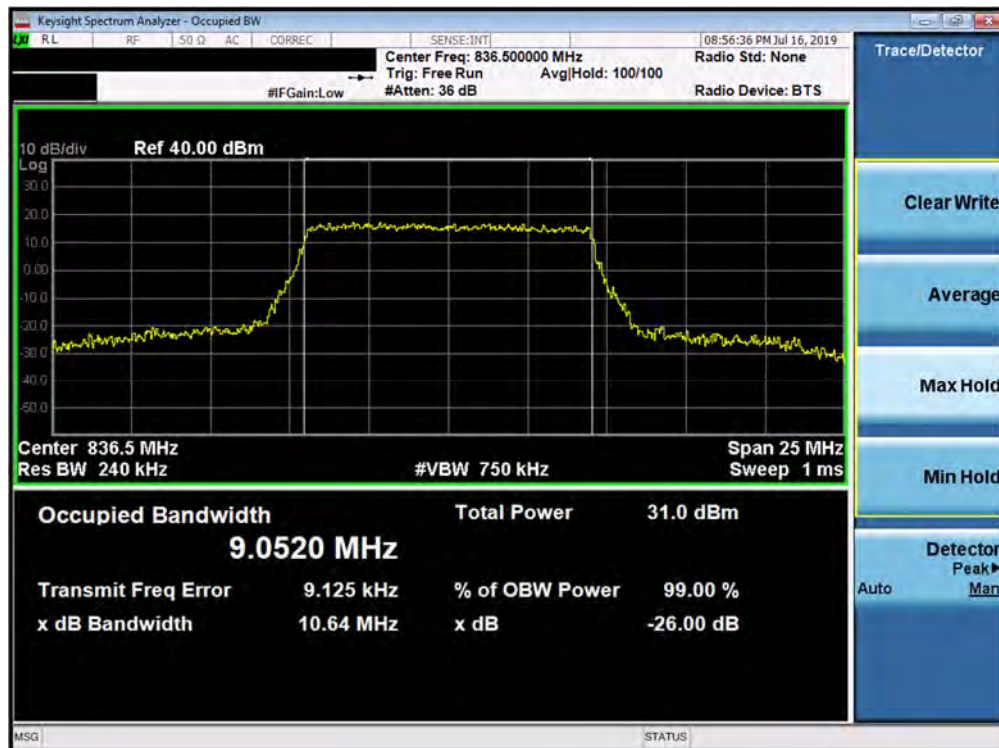
Plot 7-8. Occupied Bandwidth Plot (Band 5 - 10.0MHz 16-QAM - Full RB Configuration)
