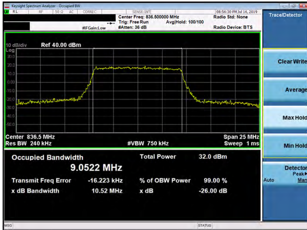
Plot 7-7. Occupied Bandwidth Plot (Band 5 - 10.0MHz QPSK - Full RB Configuration)
