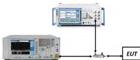
Figure 7-2. Test Instrument & Measurement Setup
