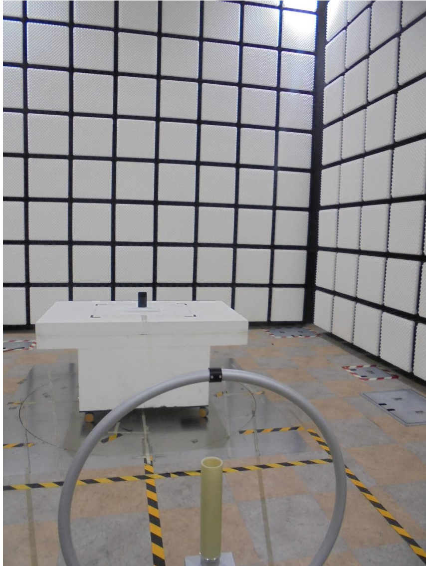
NFC Radiated Test Setup Photo for below 30 MHz:
