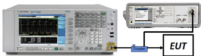
Figure 7-4. Test Instrument & Measurement Setup
