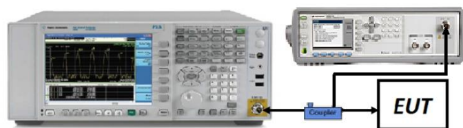
Figure 7-5. Test Instrument & Measurement Setup
