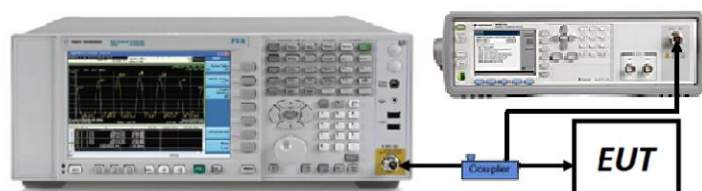
Figure 7-7. Test Instrument & Measurement Setup
