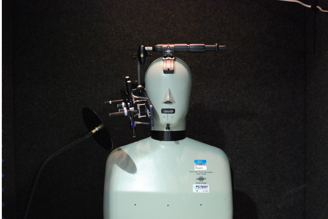
Figure 17-1 Test Setup for Wireless Device
