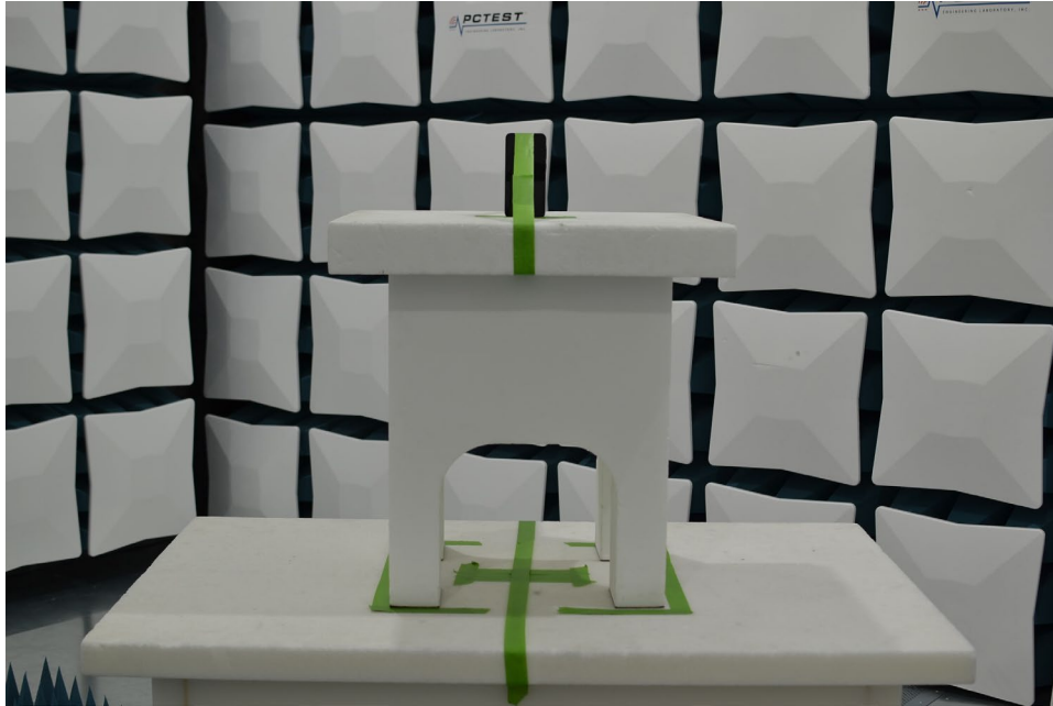
Figure 3. Test Setup – Z Position – 1GHz-18GHz
