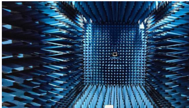
Figure 2: Geometry of Anechoic Chamber for Radiation patterns.
