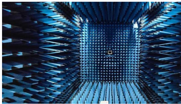
Figure 2: Geometry of Anechoic Chamber for Radiation patterns.
