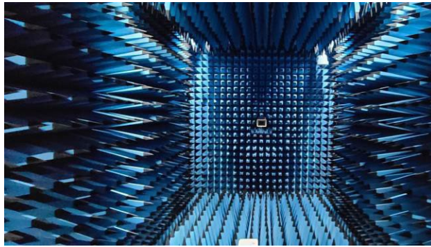
Figure 2: Geometry of Anechoic Chamber for Radiation patterns.
