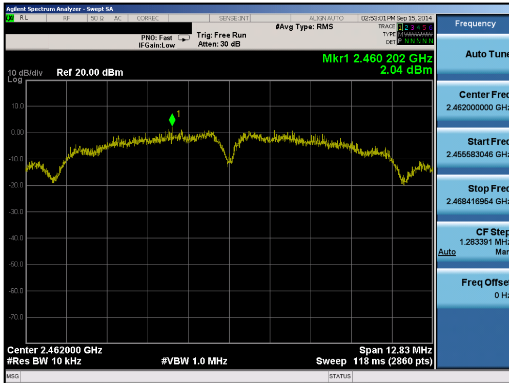
Plot 6-20. Power Spectral Density Plot (802.11b – Ch. 11)
