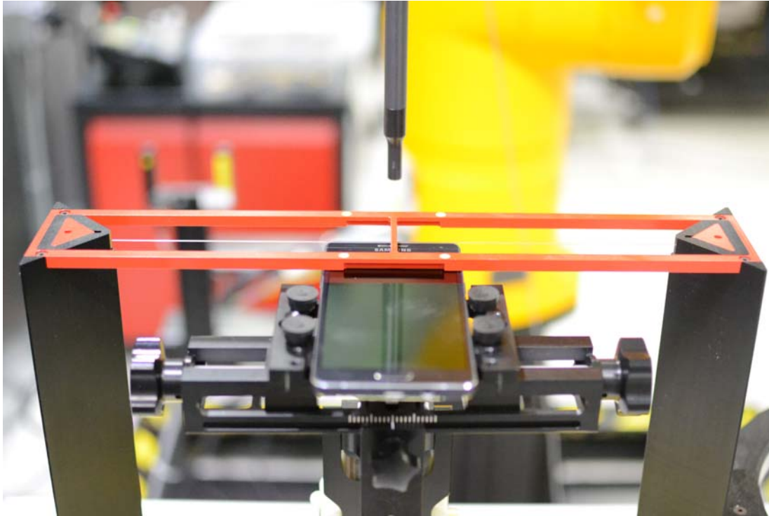
Figure 18-1 Ear Reference Point HAC Phantom Alignment
