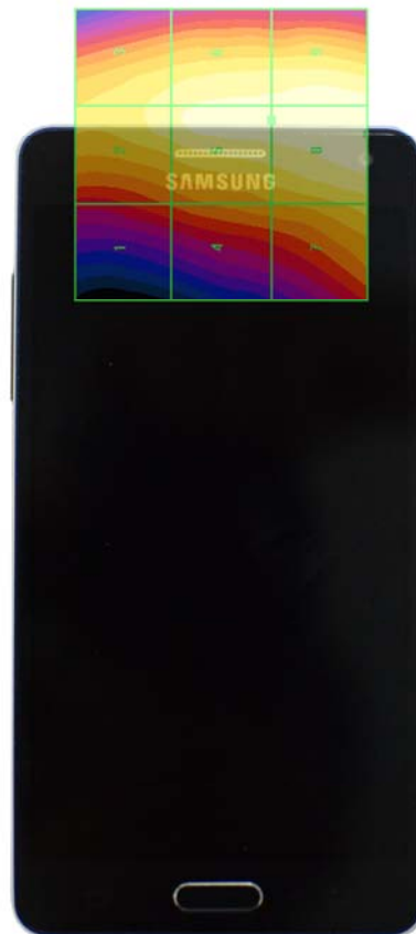
Figure 18-4 E-Field WD Scan overlay
