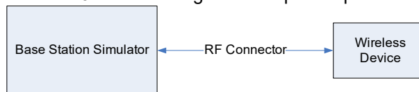
Figure 9-3 Power Measurement Setup
