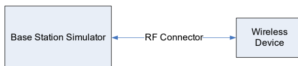
Figure 9-1 Power Measurement Setup
