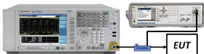
Figure 7-3. Test Instrument & Measurement Setup
