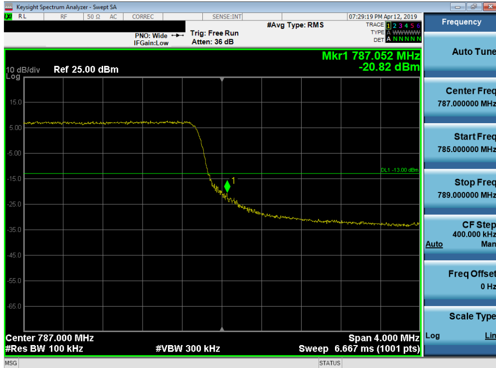
Plot 7-213. Upper Band Edge Plot (Band 13 - 5.0MHz QPSK - Full RB Configuration)
