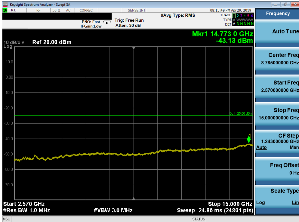
Plot 7-170. Conducted Spurious Plot (Band 7 - 20.0MHz QPSK - RB Size 1, RB Offset 0 - Mid Channel)
