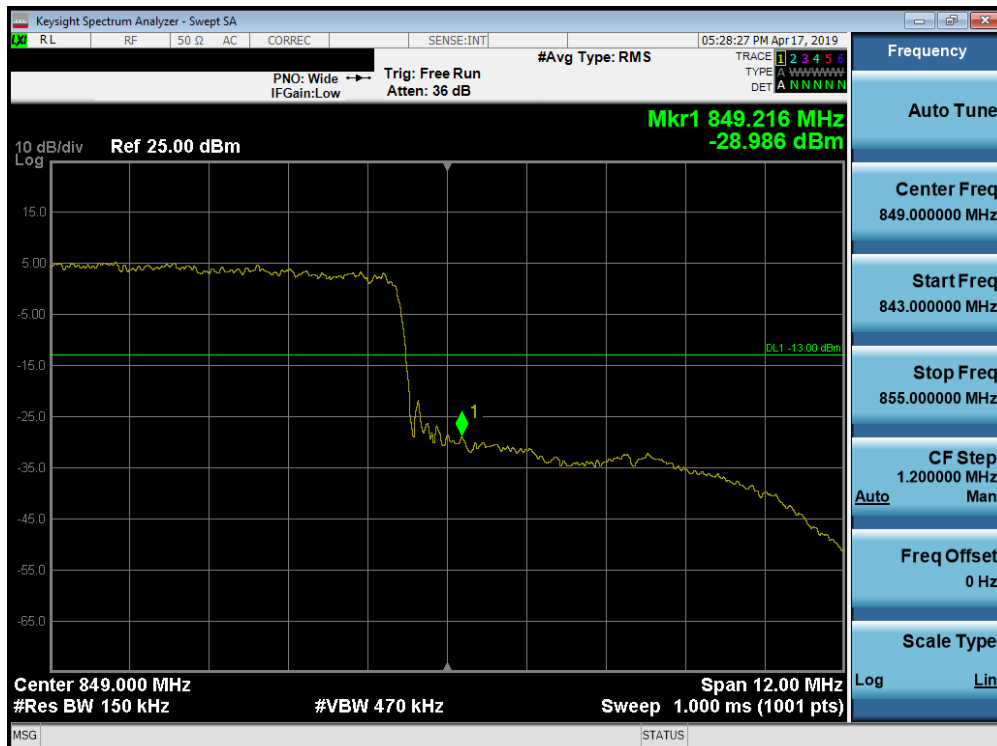
Plot 7-228. Upper Band Edge Plot (Band 26 - 15.0MHz QPSK - Full RB Configuration)
