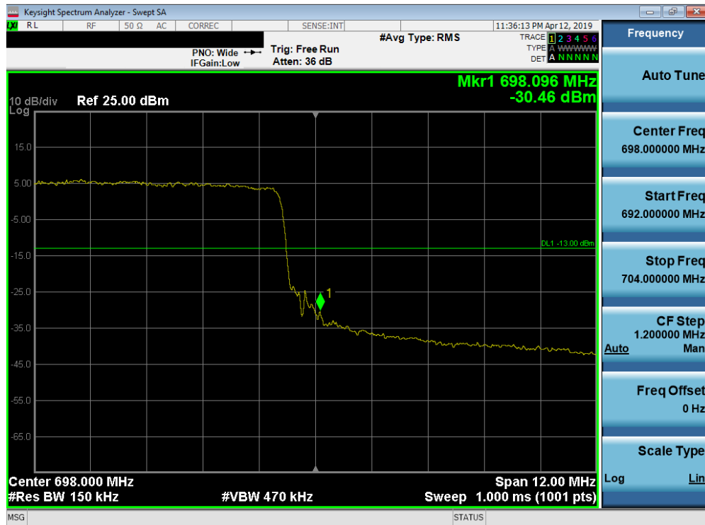
Plot 7-198. Upper Band Edge Plot (Band 71 - 15.0MHz QPSK - Full RB Configuration)
