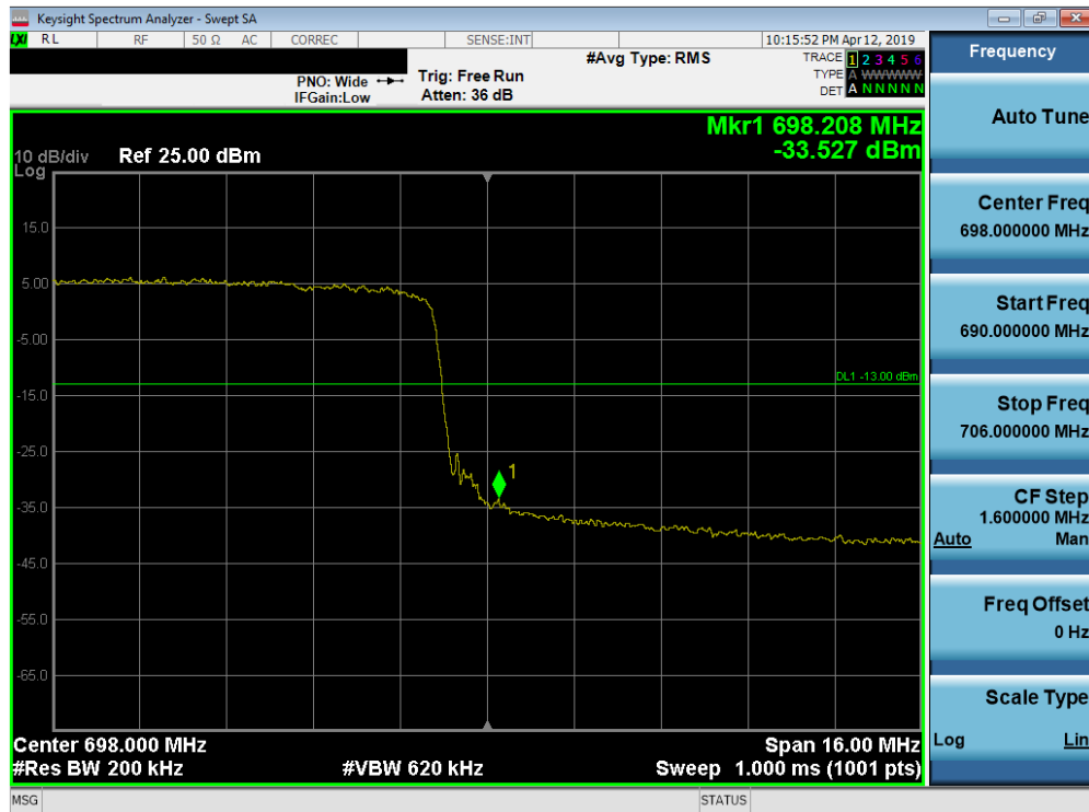
Plot 7-200. Upper Band Edge Plot (Band 71 - 20.0MHz QPSK - Full RB Configuration)
