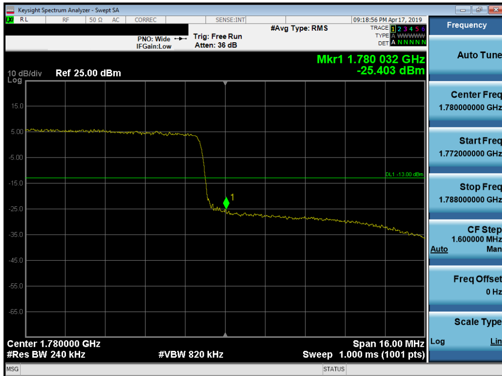
Plot 7-263. Upper Band Edge Plot (Band 66 - 20.0MHz QPSK - Full RB Configuration)
