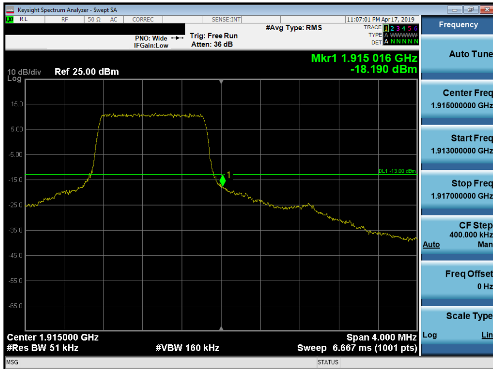
Plot 7-269. Upper Band Edge Plot (Band 25 - 1.4MHz QPSK - Full RB Configuration)
