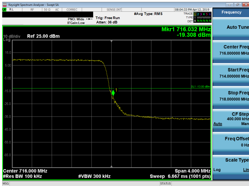
Plot 7-204. Upper Band Edge Plot (Band 12 - 3.0MHz QPSK - Full RB Configuration)
