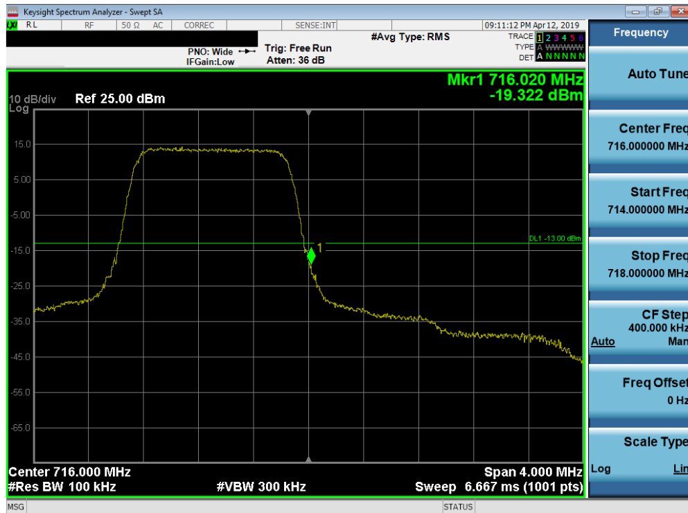
Plot 7-202. Upper Band Edge Plot (Band 12 - 1.4MHz QPSK - Full RB Configuration)
