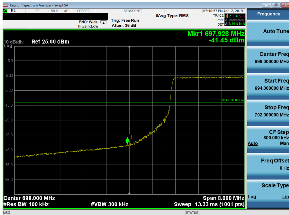
Plot 7-208. Lower Band Edge Plot (Band 12 - 10.0MHz QPSK - Full RB Configuration)
