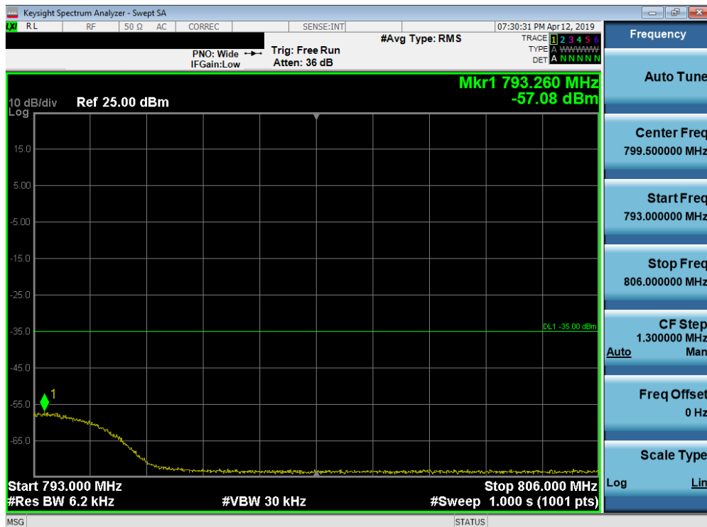
Plot 7-214. Upper Emission Mask Plot (Band 13 - 5.0MHz QPSK - Full RB Configuration)
