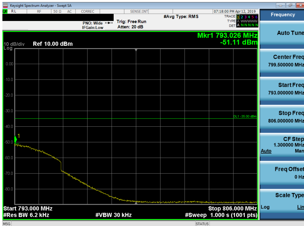
Plot 7-218. Upper Emission Mask Plot (Band 13 - 10.0MHz QPSK - Full RB Configuration)
