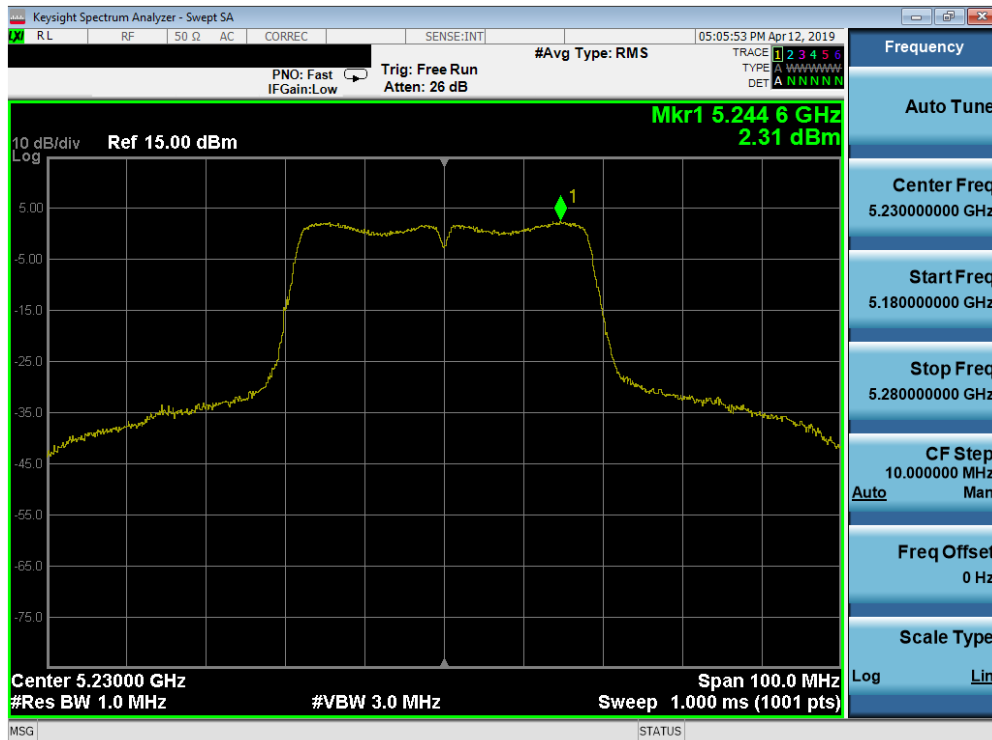
Plot 7-47. Power Spectral Density Plot (40MHz BW 802.11n (UNII Band 1) – Ch. 46)
