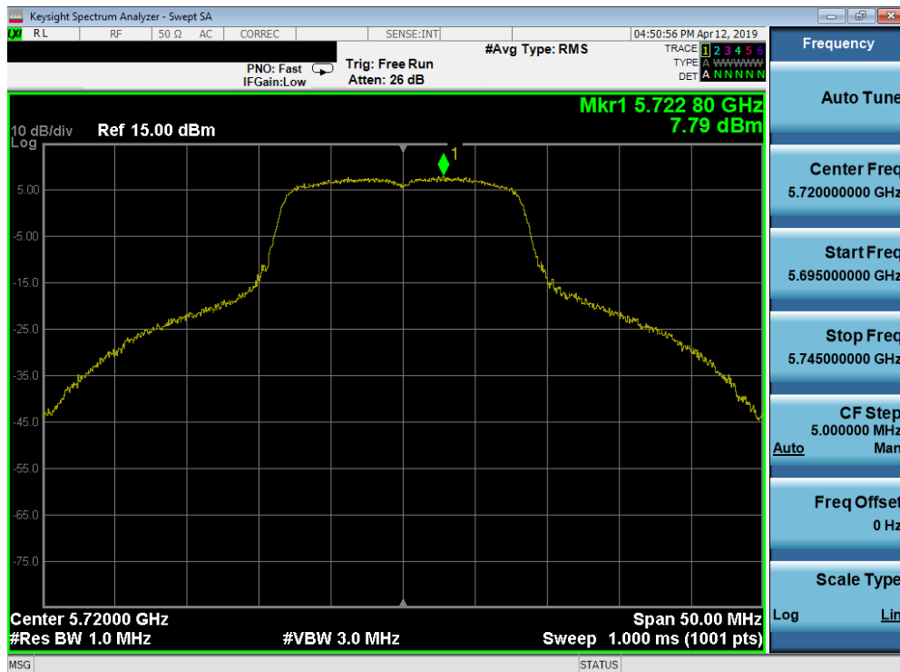
Plot 7-60. Power Spectral Density Plot (802.11a (UNII Band 2C) – Ch. 144)
