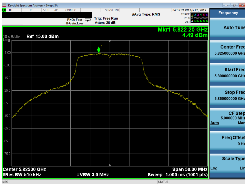
Plot 7-72. Power Spectral Density Plot (802.11a (UNII Band 3) – Ch. 165)
