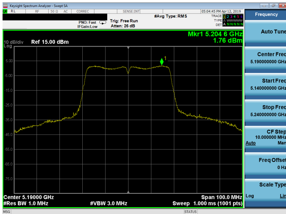
Plot 7-46. Power Spectral Density Plot (40MHz BW 802.11n (UNII Band 1) – Ch. 38)
