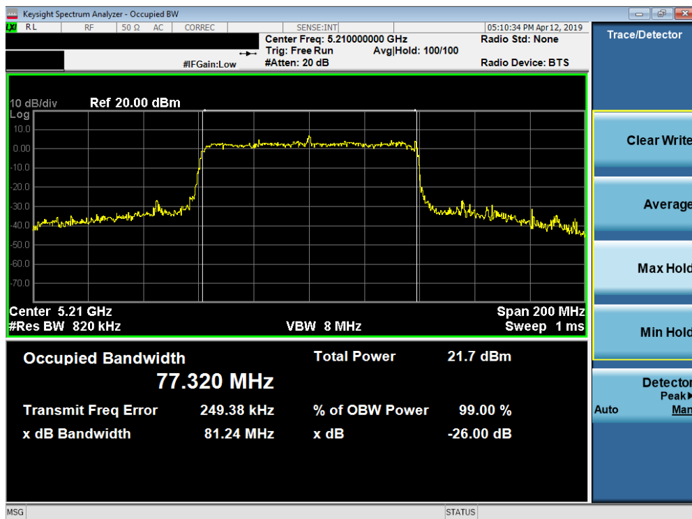
Plot 7-9. 26dB Bandwidth Plot (80MHz BW 802.11ac (UNII Band 1) – Ch. 42)
