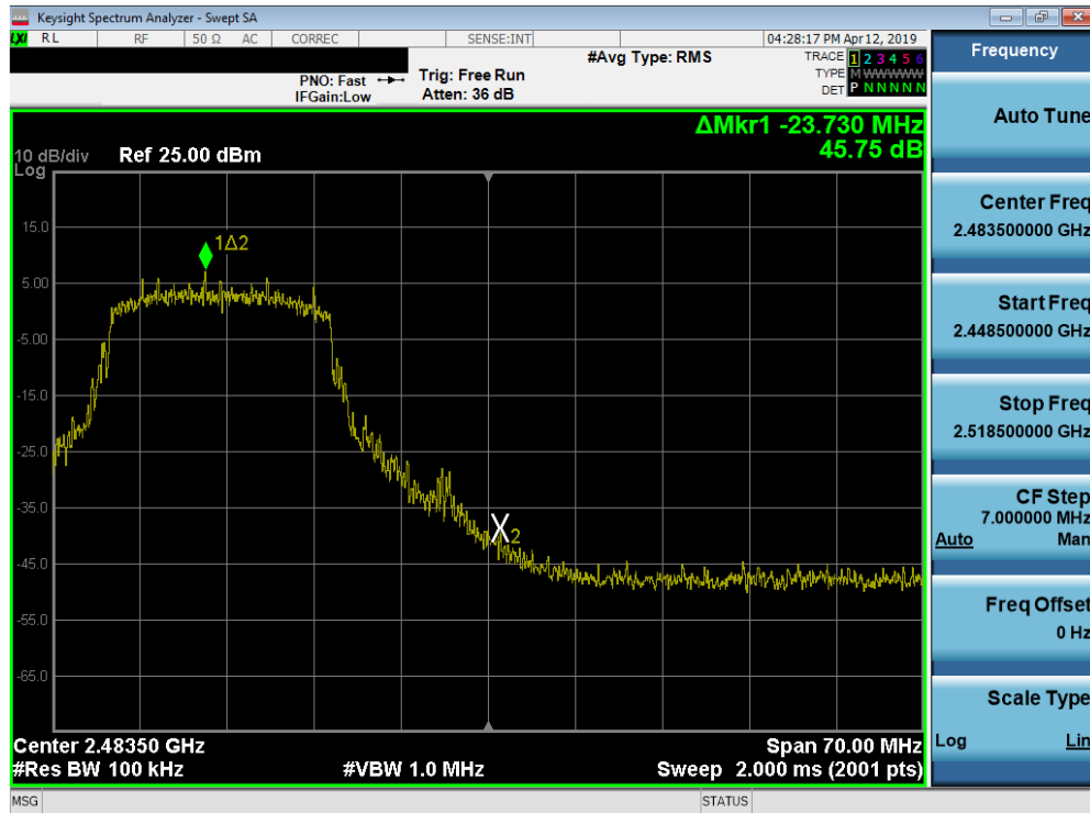
Plot 7-29. Band Edge Plot (802.11n – Ch. 12)
