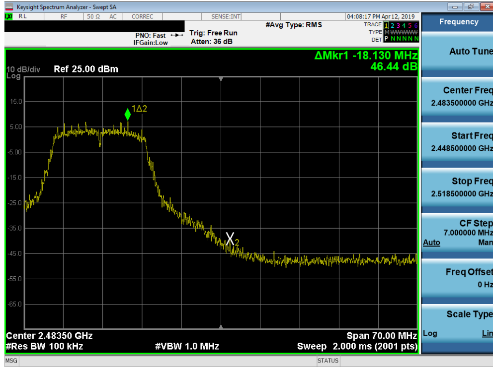
Plot 7-25. Band Edge Plot (802.11g – Ch. 12)
