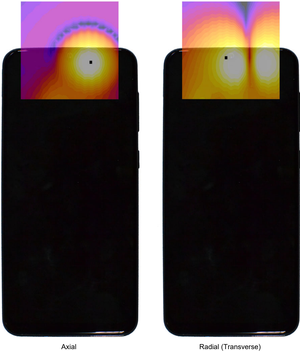
Figure 16-3 T-Coil Scan Overlay Magnetic Field Distributions
