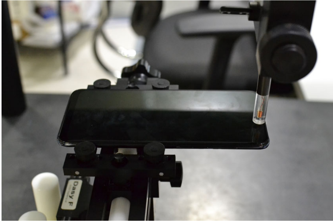
Figure 16-1 Test Setup for Wireless Device
