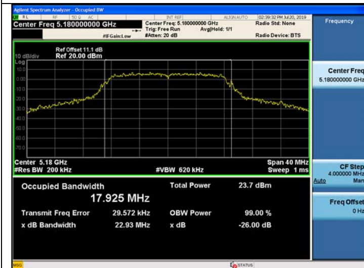
802.11a UNII 2C BAND 26dB Bandwidth (CH120)
