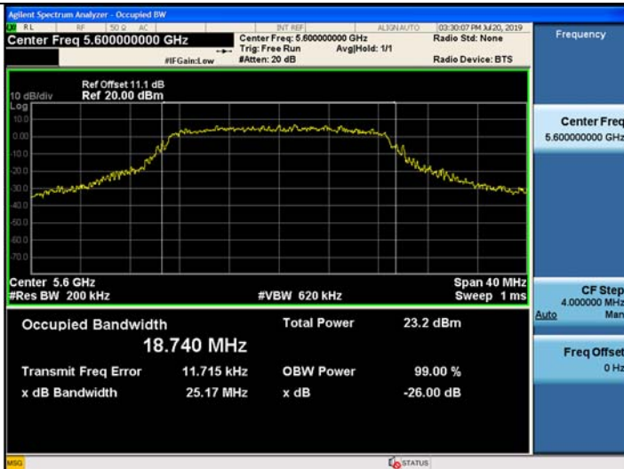
802.11ac_VHT20 UNII 2C BAND 26dB Bandwidth(CH 120)
