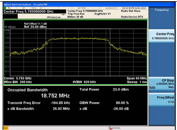
802.11n_HT20 UNII 3 BAND 26dB Bandwidth(CH 157)
