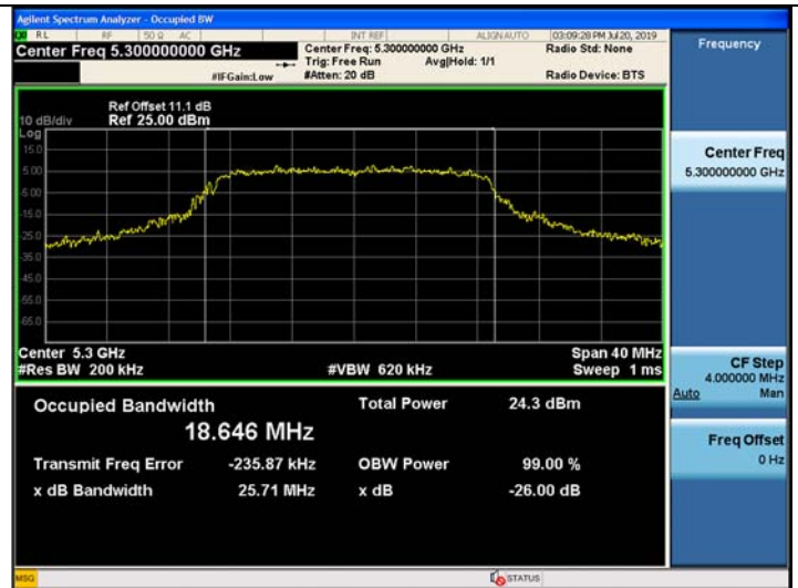
802.11n_HT20 UNII 3 BAND 26dB Bandwidth(CH 157)
