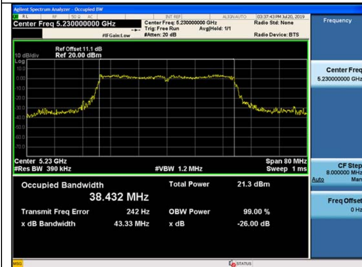
802.11n_HT40 UNII 2C BAND 26dB Bandwidth(CH 102)
