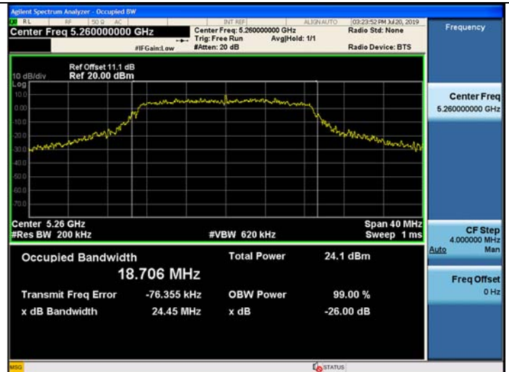
802.11ac_VHT20 UNII 3 BAND 26dB Bandwidth(CH 149)
