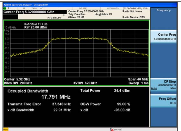
802.11a UNII 3 BAND 26dB Bandwidth (CH 157)
