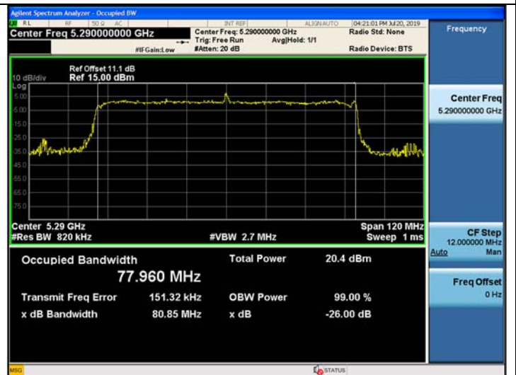
802.11ac_VHT80 UNII 3 BAND 26dB Bandwidth (CH 155)
