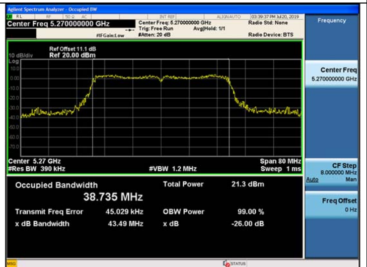
802.11n_HT40 UNII 3 BAND 26dB Bandwidth (CH 151)
