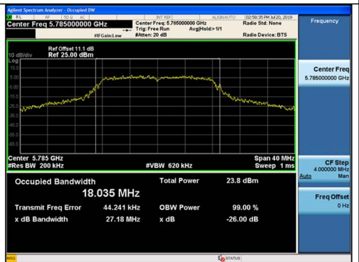
802.11a UNII 3 BAND 26dB Bandwidth (CH 157)
