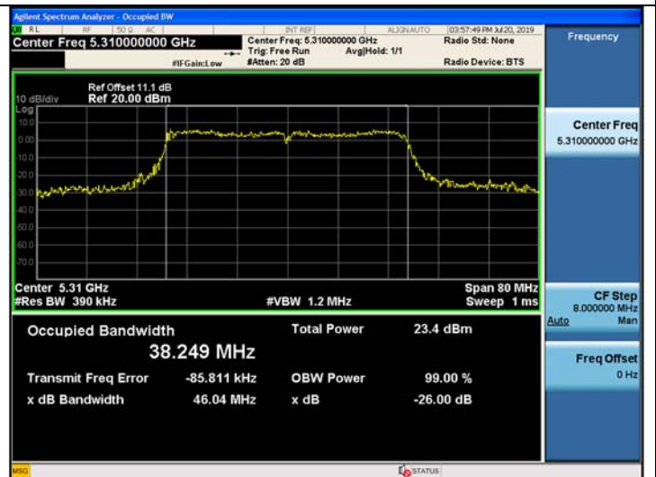
802.11ac_VHT40 UNII 3 BAND 26dB Bandwidth (CH 159)
