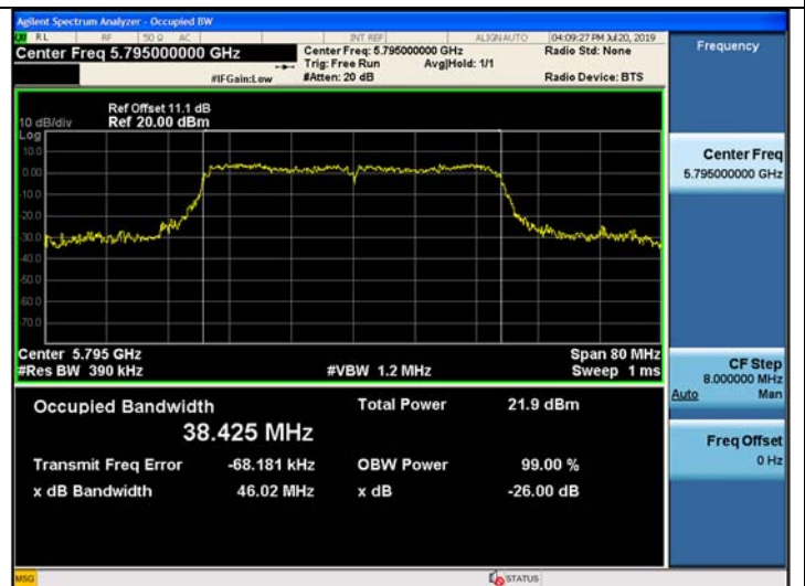
802.11ac_VHT40 UNII 3 BAND 26dB Bandwidth (CH 159)
